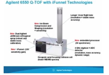
So, typically like in a quadruple time of flight instrument, you have a quadrupole and then a time of flight where the ions will travel like this and time is measured coupled with collision cell where you trigger an MS/MS. When we say what is the word we typically use, LC-MS/MS, okay. So, there is a LC component, liquid chromatography component also coupled to an MS, okay. Why so, because we want to separate.
