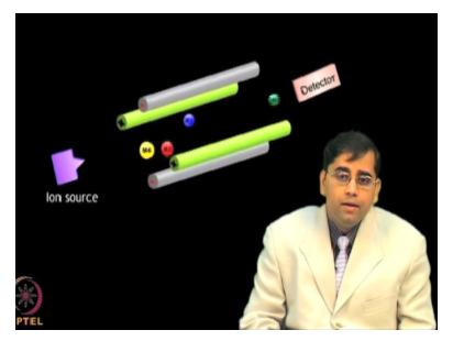
Quadrupole, it consists of four parallel metal rods and mass separation is accomplished by the stable vibratory motion of ions in a high frequency oscillating electric field that is created by applying direct current and radio frequency potentials to these electrodes.
