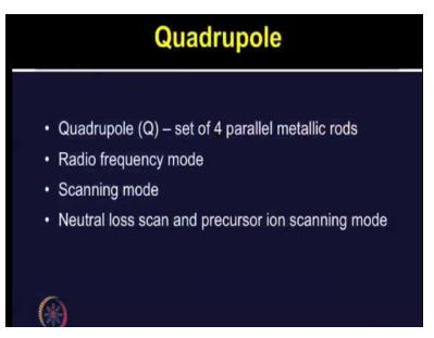
So as talked Quadrupole is set of 4 parallel metallic rods with opposite players electrically connected. The different modes one can use of this analysis RF or radio frequency mode which allows ions of any M/Z ratio to pass through scanning mode, ions of selected mass by charge can be allowed by the detector the potential difference applied and instrument can be used as a mass filter.
