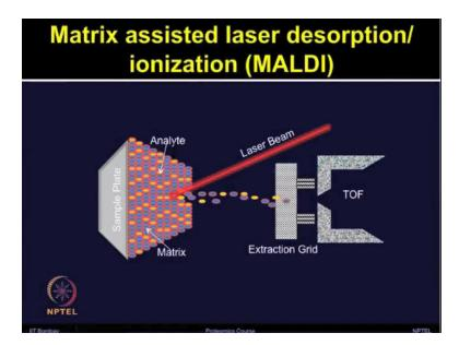
The ionization source is responsible for converting analyte molecules into gas phase ions in vacuum.
