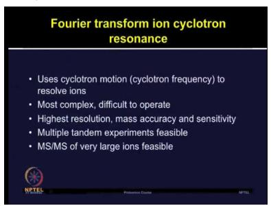
And FT-ICR MS can be considered as an ion trap system where ions are trapped in the magnetic field. It uses cyclotron motion or cyclotron frequency to resolve the ions, although operationally it is complex and not really to operate but it provides highest resolution mass accuracy and
