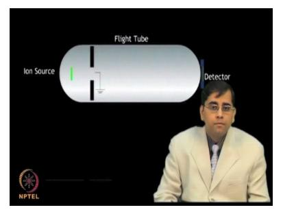
The Time-of-Flight measured M/Z ratio of ions based on the time it takes for ions to fly in the analyzer and strike to the detector.
