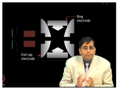
The Ion Trap, it traps ions using electrical fields and measures mass by selectively ejecting them to rejecter.
