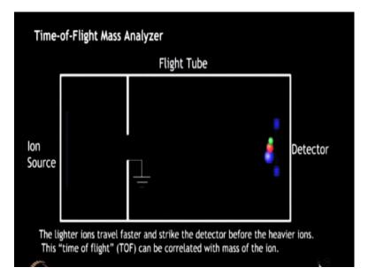
The Time-of-Flight Mass Analyzer resolves ions produced by the ionization source on the basis of their mass to charge ratio. The Time-of-Flight tube can be operated in the linear mode or the reflectron mode which depends on the sample to be analyzed. In case of a small molecules this mode usually provides sufficient resolution. The generated ions are accelerated towards the detector with the lighter ion travelling through the TOF tube faster than the heavier ions.
