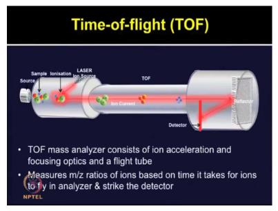
So the TOF mass analyzers, they consist of ion acceleration and focusing optics and a flight tube. As shown in the slide, you have source, the sample ionization is occurring due to the laser beam bombardment then ions are moving in the time-of-flight tube and reaching towards the detector. Now often we can also add the refractor and ion mirror which can increase the path length.
