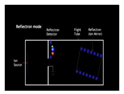
So this is more commonly use for the proteomics studies. A reflectron which acts as a ion mirror it is incorporated at one end of the Time-of-Flight tube. This helps in extending the path length and in turn the flight time of the ion without having to increase the actual size of the instrument. So rather than using very long Time-of-Flight tube by including the reflectron ion mirrors, we can increase the path length.
