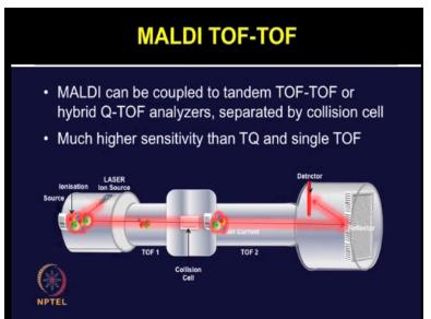
MALDI TOF-TOF that is one of the widely used tandem MS configuration. In this one the TOF-TOF or two time-of-flight tubes as well as hybrid Quadrupole time of flight analyzers can be used. We have discussed the MALDI TOF-TOF system in some more detail in the previous lecture. Shall move onto some other configurations which is Q-TOF.
