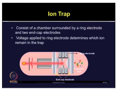
The Ion Trap, traps ion using electrical fields and it measures by selectively ejecting them to a detector. It consists of a chamber which is surrounded by a ring electrode and two end-cap electrodes as you can see in this figure here. The voltage applied to the ring electrode determines which ion remain inside the trap. So ions above a threshold of M/Z ratio they remain inside the trap and others can be ejected through the small hole.
