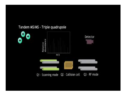
The Triple quadrupole consists of two sets of parallel metallic rods intersperse by a collision cell. The first quadrupole scans the ions coming from the ionization source and allow only ions of a particular M/Z ratio to pass through. Once ions are selected these ions enter the collision cell where they are fragmented by collision against an inner gas like argon.
