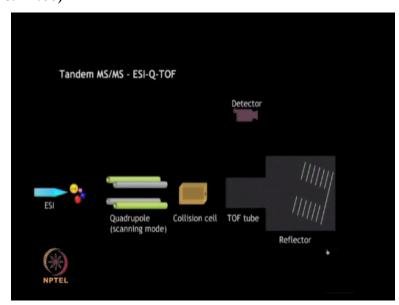
ESI-Q-TOF is another common tandem MS configuration that first selects ions in radio frequency mode. Selected peptides are fragmented in collision cells and resulting ions are accelerated and resolved on the basis of the time of flight.
