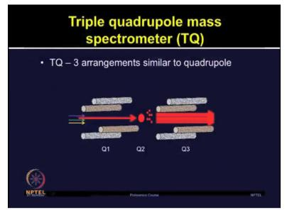
Now Triple quads, which is arrangement of Quadrupoles is widely use for the proteomics. In triple quad the Q1 scans ions it streams, it direct ions of a selected M/Z ratio into the second quadrupole, Q2 which is the collision cell. As you can see in this slide the collision cell operates in the radio frequency mode, the fragmentation of intact peptide ions can be induced by colliding with inured gases and then selected ions are further moved into the Q3.
