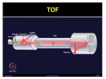
In TOF, the ions are accelerated to high kinetic energy and due to their different velocities they are separated in a flight tube. One can also use the reflectron mirror so that ions can turnaround into a reflected and it can compensate for minor differences in the kinetic energy and provide long separation. Another commonly used mass analyzer is Quadrupole. The instruments are one of the most widely used type of mass analyzers currently used in proteomic.
