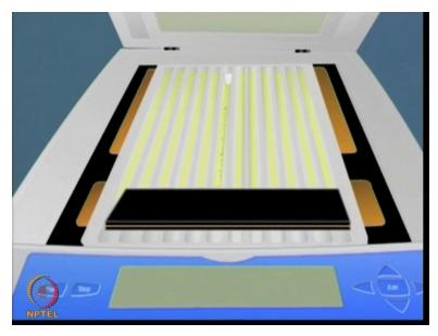
So, remove the IPG strip from the cover place it in the rehydration tray. Add the reconsidered protein sample on this strip. Pour mineral oil to prevent it from the dry and then move forward for the isoelectric focusing. So, place the width and ideal length of the IPG strip followed by an electrode at each end fill all the adjacent dwells with the mineral oil to ensure the uniform current flow.
