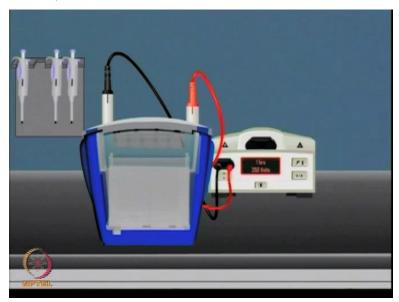
When the gel is polymerized then you can add the IPG strip and now ensure that assembly is properly sealed, and buffers are properly placed. So, that proteins can be separated based on their molecular weight depending on the gel length you can perform the second-dimension separation for a few hours.
