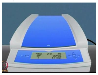
You can input the desired protocol on the instrument software along with the details of its strip length pH range number of its strip etc. and to start the focusing process.
