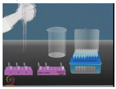
So, prepare the Bradford reagent and label the tube suitably for the standard and test samples add the standard and sample solutions to their respective tubes. Now add the Bradford color reagent to the tubes and mix them thoroughly.
