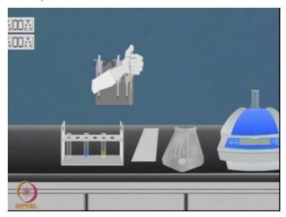
Once you obtain good amount of proteins which will determine by the protein quantification. Now proceed for the rehydration of immobilized pH there in the strips and focusing of these rehydrated strips.
