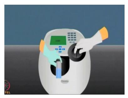
Once the color reaction has occurred then perform the absorbance measurement at 595 nanometers.
