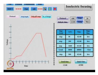
You can monitor the focusing progress on the software and you need to ensure that focusing is proper. During the IEF proteins will migrate along the strip and come to rest at a point when their net charge become 0 which is known as their Isoelectric point.
