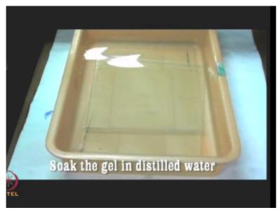
Gel removal and protein fixation soak; the gel present between the glass plates in fresh distilled water to remove any bound SDS.
