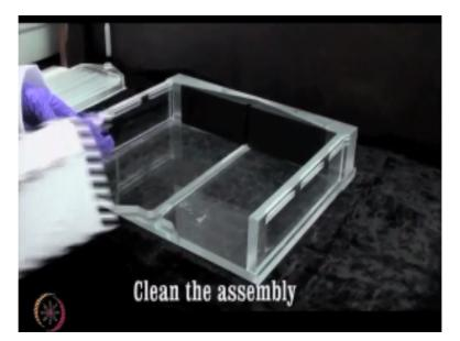
Assembly of gel apparatus and gel casting; clean all the components of the gel assembly thoroughly with water and dry them with paper towels.
