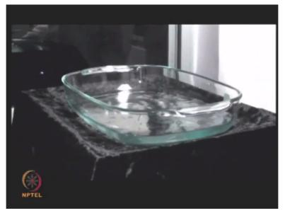
Place the tray on a mechanical shaker for an hour to ensure that the protein spots get fixed onto the gel thereby minimizing any diffusion.
