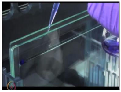
Then pour the lukewarm agarose overlay solution over the strip to prevent the gel from drying up.
