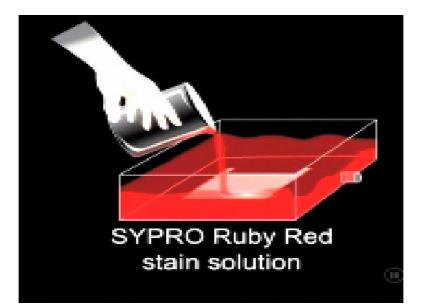
After fixation a step, the gel is soaked in the fluorescent SYPRO Ruby red stained solution. (Refer Slide Time: 19:49)
