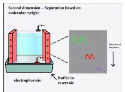
The proteins having lower molecular weights have high mobility and migrate further through the gel pores, while the high molecular weight proteins remain closer to the point of application. This allows efficient separation of the proteins in the second dimension.
