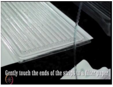
SDS page; drain out the excess liquid of the second equilibration solution from the IPG strip using a tissue paper.
