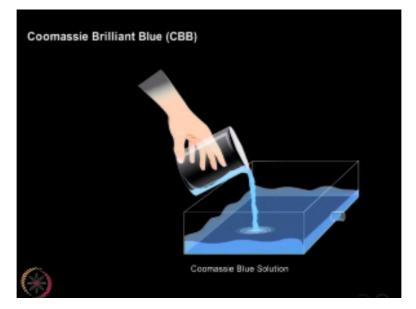
The biosafe Coomassie is also ready to use a stain and a single reagent protein stain, so I will show you one animation, how to perform the Coomassie blue staining. In this animation, I will show you how the staining can be performed by using Coomassie brilliant blue stain. The completed electrophoresis gel is placed in a tray containing the Coomassie blue a staining solution typically are 250, that has been dissolved in an eco-solution of methanol and acetic acid.
