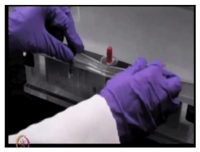
Close the casting assembly and tighten the screws provided.
