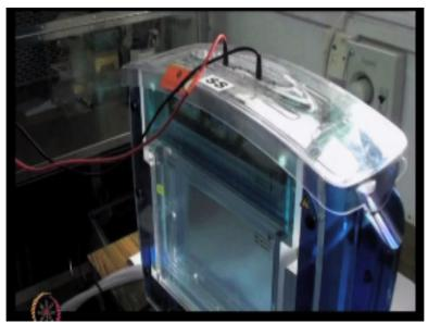
Close the gel assembly and connect the apparatus to the electricity supply, set the appropriate voltage and begin the run.
