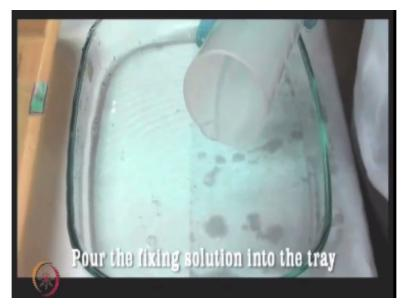
Pour the fixing solution containing methanol and acetic acid into another tray. (Refer Slide Time: 30:22)
