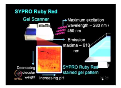
The MS compatible gel is then viewed using UV or laser scanning instrument with an excitation wavelength near 280 or 450 nanometres. This stain has 2 excitation maxima and emission maxima of 610 nanometre. In this animation, you can see a gel pattern, which is showing you the staining obtained after SYPRO Ruby red and it is showing separation in 2 dimension based on the molecular weight and isoelectric point.
