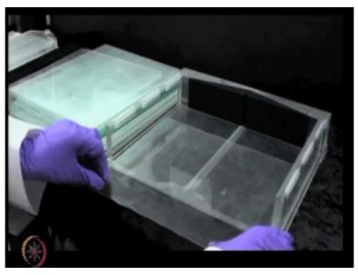
Carefully arrange the glass plates in the gel casting assembly interspersed with separator sheets depending on the number of gels to be run. The assembly should be tightly packed such that there are no leaks.
