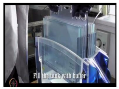
Assemble the remaining plates in the gel assembly and carefully lowered the entire apparatus into the gel tank containing the buffer solution, ensure that the buffer level does not rise above the mark indicated.
