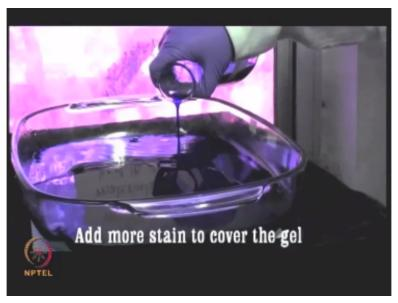
Add some more staining solution such that the gel is completely immersed and leave it overnight for around 8 to 10 hours.
