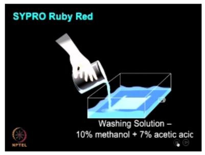
After this overnight, the step of staining; the gel can be washed with methanol and acetic acid solution.
