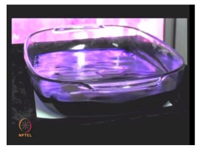
Gel staining transfer the gel carefully into another tray containing the Coomassie blue staining solution and place it on the shaker to ensure uniform contact of the gel with the solution.
