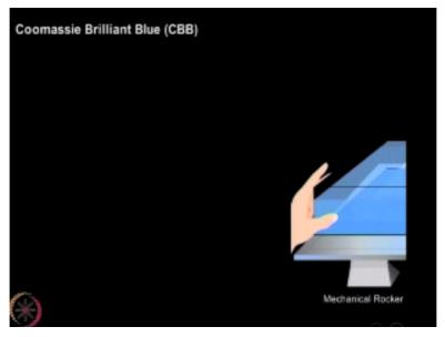
After adding the stain, the tray is then placed on a mechanical rocker, which allows for uniform contact of the gel with the solution by means of gentle rocking.
