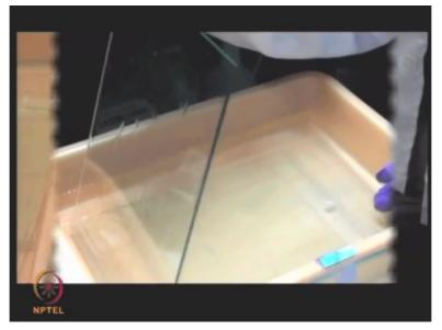
Open the glass plates and carefully remove the IPG strip from the gel.
