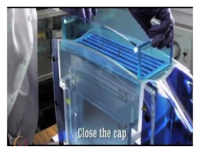
Place the separating chamber above this and pour the buffer solution into the upper chamber. (Refer Slide Time: 05:39)
