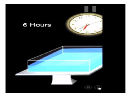
For uniformed destaining, it is good idea to keep it on gentle shaking for at least 6 hours. (Refer Slide Time: 26:45)
