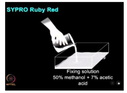
In that light, SYPRO Ruby is very compatible for mass spectrometry and you can further characterize your proteins. So, now I will show you the steps involved in performing SYPRO Ruby staining, so I will show you one animation. SYPRO Ruby red the completed gel is first placed in a fixing solution of methanol and acetic acid that fixes the protein bands in the gel and minimizes any diffusion.
