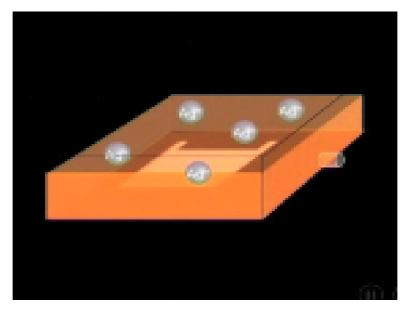
After adding the silvered solution, the gels are rock gently in order to allow for proper and uniform staining.
