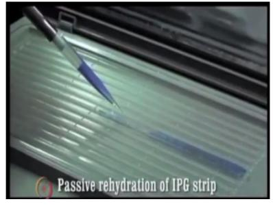
IPG strip rehydration; clean all the apparatus thoroughly before use to avoid any contamination, add the reconstituted protein sample in a well of the rehydration tray.
