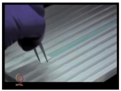
Then place the two wicks at either end of the IPG strip followed by an electrode at each end. (Refer Slide Time: 21:38)
