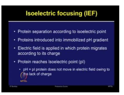
You can take the immobilise pH gradient strip and apply the protein solution on the IPG strip, so that protein is absorbed on the strip and then after applying the electric field, the proteins will migrate according to its charge. When protein is reaching to its isoelectric point, where pH becomes equal to isoelectric point or PI, then proteins do not move in the electric field because of the lack of charge.
