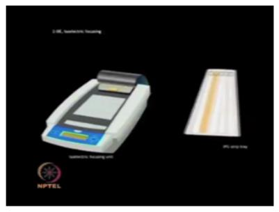
This is then placed in the isoelectric focusing instrument and low voltage is applied. (Refer Slide Time: 05:32)
