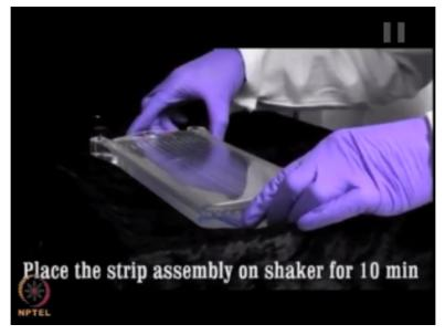
Place the assembly on a mechanical shaker for 10 minutes.
