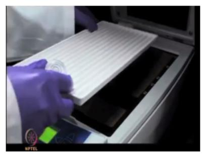
Isoelectric focusing; initialize the instrument and clean the surface well with a dust free cloth, place the focusing tray on the instrument and ensure that it is properly balanced.
