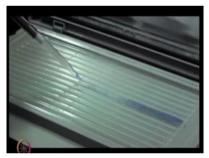
Place the third IPG strip in the tray and over it, pour the first equilibration solution consisting of urea, Tris-HCL of ph 8.8 glycerol SDS bromophenol blue along with dithiothreitol or DDT. (Refer Slide Time: 29:17)
