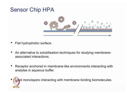
Another very important and variety of chip surface is HPA surfaces are flat hydrophobic surfaces and these surfaces are useful for membrane associated interactions. Receptors generally are anchored into a membrane-like environments and then they are useful for interaction with analytes. Generally, the lipid monolayers interacting with membrane binding bio-molecules kind of studies are made on these surfaces.
