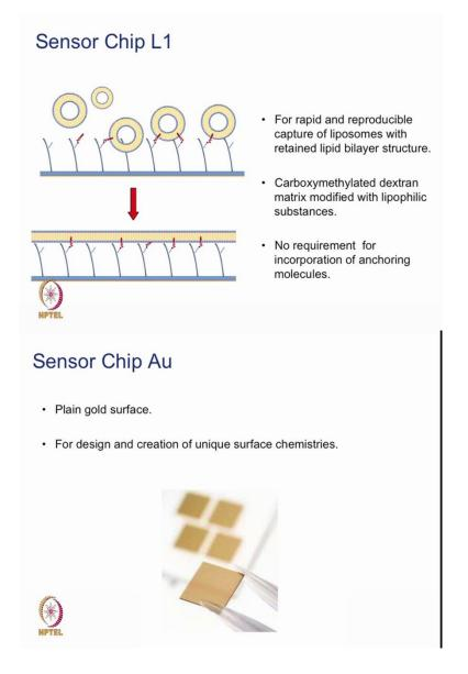
L1 another surface sensor chip, which is also popularly used for studying liposomes, lipid bilayer kind of a molecules and carboxymethylated dextran is modified with lipophilic substances. So, another surface is a plain gold surface where there will not be any dextran and these surfaces are very good with chemists where they can do their own chemistries and useful for interaction.
