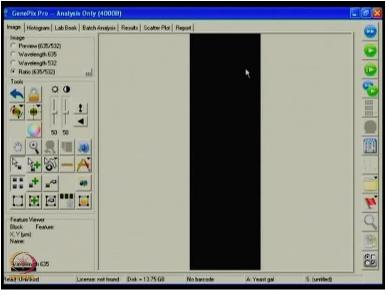
Mr. Pankaj Khanna: So, what you see now is a GUI or graphical user interface of genepix pro software. On top it is in the form of different tab buttons which allows you in different work group say for example image allows you in different ways and controlling of the image acquisition and histogram looks at how that image has performed. So this is what we were speaking about in the earlier slide where we can see a live kind of demo which is happening.
