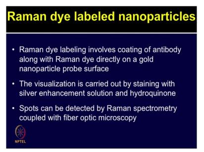
The Raman dye labeling involves coating of antibodies on the array surface like gold by using the Raman dye directly on the gold surface which are in nanoparticles probes. The visualization can be carried out by staining with silver enhancement solution as well as hydroquinom. Spot can be detected by Raman spectrometry coupled with fiber optic microscopy.
