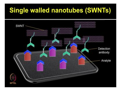
The macromolecular single walled Nano tubes SWNTs functionalized with a specific Raman dye neighbor antibodies are used for multiplexed detection target proteins bound on the microarrays slide, which is gold coated. As you can see this slide SWNT functionalized with Raman dye labeled antibodies are used for multiplexed detection of target proteins which are bound on the gold coated microarray surface.
