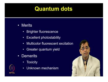
Key advantages of quantum dots compare to the organic dyes include its brighter fluorescence, excellent photostability, multicolour fluorescent excitation and higher quantum yield. Despite of several benefits and applications in a variety of biological sample and demerits includes toxicity. Therefore, quantum dots have shown various applications but the still they have certain limitations. We will talk some of these applications during the course of interactomics molecules.
