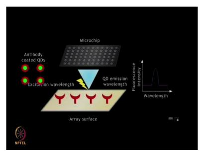
So, as you can see upon binding of the target protein to the antibody. Now, these changes are plotted on the wavelength verses florescence intensity graph. So these quantum dots can detect molecules with very high sensitivity in femtomolar range.
