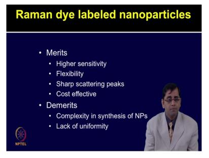
As compared to the fluorescence based detection methods the Raman dye labeled, gold Nano probes offers several advantages which include high sensitivity, flexibility due to non-overlapping probes, sharp scattering peaks and cost effectiveness of the assays. However, the
