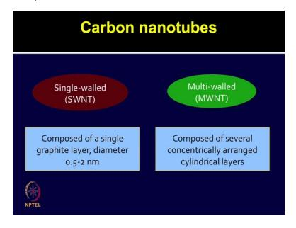
There are two different types of carbon Nanotubes, single walled Nanotubes SWNT, and multi walled Nanotubes MWNT. The single walled Nanotubes are composed of single graphite layer with a diameter in the range of point 5 to 2 nanometre. Whereas the multi walled Nanotubes are composed of seven concentrically arranged cylindrical layers. There are various properties associated with each of this group. Today we will focus more on how these Nanotubes can be applied for Proteomic applications.
