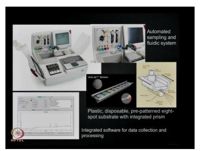
Okay, so here is the instrument, it is so computerised pumping system software, and it has little sample cell that has 9 parts that you can put down different proteins or different snippets of DNA whatever biomolecule you are trying to assay.
