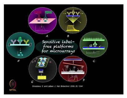
But some of the label free techniques shown here are very promising for high throughput protein microarrays or DNA microarrays based applications. As you can see in the panel A on top is based on Raman labels based on multicoloured single bond Nano tubes, tag for the multiplexed protein detection. The Panel B is Surface Plasmon Resonance which measures change in the reflective index along with the sensogram which is shown in the bottom of the same image.
