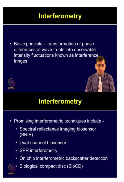
We have already discussed about SPR imaging based technique, ellipsometry based techniques, and so now we will talk about interference based techniques. Let us first talk about interferometry, interference based detection techniques are powerful tool for bio chemical, and functional analysis of proteins. Its basic principle is transformation of phase differences of wave fronts into observable intensity fluctuations knows as interference fringes.
