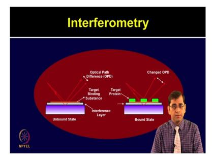
Let us look at interferometry principle in detail here. Interferometry the phase difference of wave fronts are transformed into observable intensity fluctuations which is known as interference fringes. The interferometry techniques relate the optical phase to bio molecular layer density on the surface. The signal is created by attached phase shift or optical paths difference which is caused by the absorbate bio layer.
