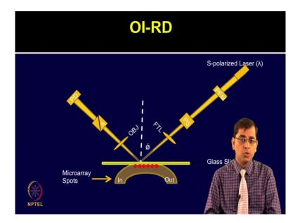
Let us talk about Oblique Incidence Reflectivity Difference or OIRD. OIRD is a form of polarization modulated imaging ellipsometer in which the harmonics of modulated photo currents are measured under the suitable nulling conditions. It can be used for label free High throuput detection of bio molecular interactions on DNA as well as protein microarrays.
