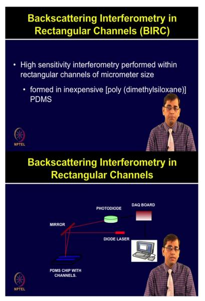
One of the interferometry technique is BIRC, or Backscattering Interferometry in rectangular channels. Let us briefly discuss this technique. This is highly sensitive interferometry approach performed within rectangular channels of micro meter size which are formed in inexpensive PDMS printed on surface.
