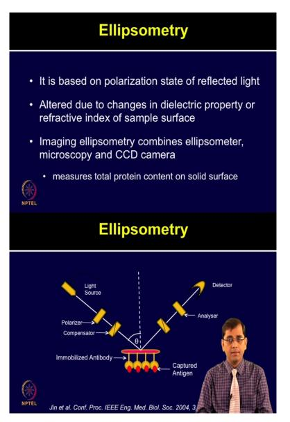
Ellipsometry is based on polarization state of the reflected light which is altered due to the changes in the dielectric property or refractive index of the sample surface. The imagining Ellipsometry combines ellipsometer, microscopy, and CCD camera which can measure the total protein content on solid surface.
