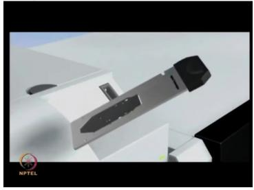
The Agilent HPLC-Chip integrates enrichment and analytical columns, micro-valve connections and
