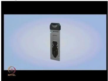
The compact architecture of the Agilent HPLC-Chip reduces peak dispersion and combines all steps from sample loading to compound ionization for a seamless operation. A closer look at HPLC-Chip
