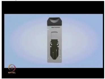
... of leaks and dead volumes and significantly improves ease of use, sensitivity, productivity and reliability. The HPLC chip also incorporates all electrical contacts
