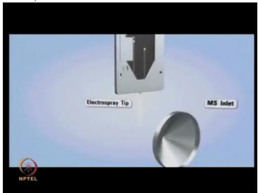
the electro spray tip orthogonal to MS inlet for maximum sensitivity and robustness
