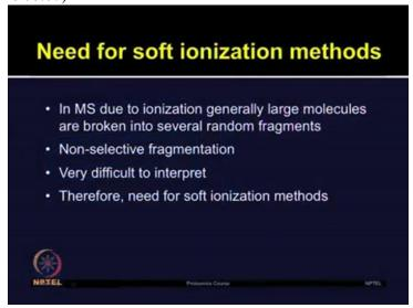
But these processes are too energy-rich to ionize intact large biomolecules and they lead to the unpredictable analyte decomposition. So for proteomic application, there was need for the soft ionization methods in mass spectrometry.
