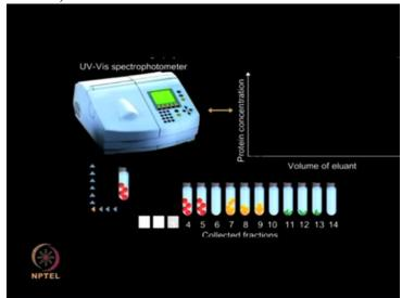
... by using a UV-visible spectrophotometer Now analyze the protein content by using UV-visible spectrophotometer at 280 nanometers. Once all the absorbance values are recorded
