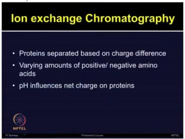
In ion exchange chromatography, the proteins are separated based on charge difference. The proteins with overall negative charge will interact with positive charges or vice versa. So, by varying the amount of positive and negative amino acids and, even pH can influence the net charge on proteins.
