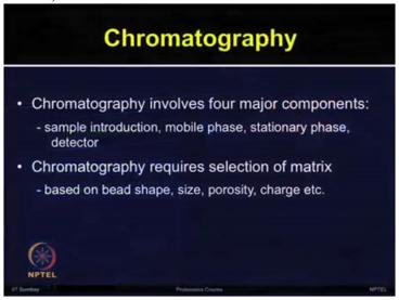
The chromatographic techniques involves four major components; an inlet for sample introduction, the mobile phase, stationary phase and a detector.
