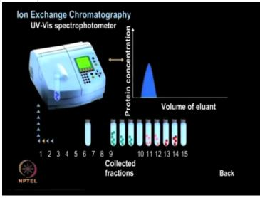
In this particular example the negative charged large molecules coming first and then positively charged fractions are coming later.
