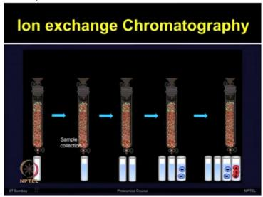
So if you have negatively charged protein which gets eluted firs will be present in the initial fractions while the positively charged protein that bound to the column will be eluted in the later fractions or it will vice versa.
