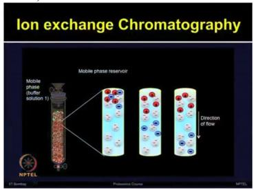
So proteins are adsorbed to the ion exchange column and then it can be desorbed by increasing the salt or altering the pH of the buffer which can change the charge on protein.
