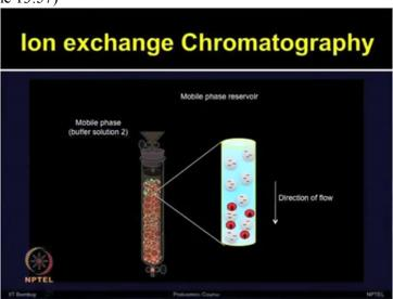
Now the buffer solution is changed so that the net pH of the protein of interest can be modified and it no longer binds to the ion exchange resin, therefore the bound protein can eluted out as shown in this slide.
