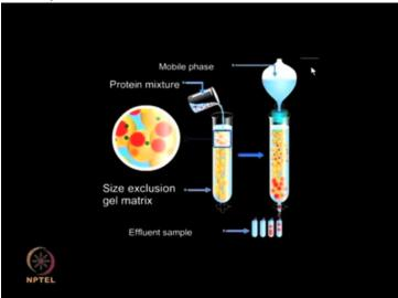
Effluent sample fractions: the solution leaving the column is collected in suitably sized fractions; initial fraction will contain only the mobile phase while later fractions will have purified proteins.
