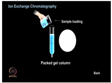
... various positively and negatively charged proteins The column is eluted with a buffer solution of suitable pH such that the negatively charged molecules are removed from the column
