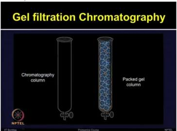
The gel filtration column is composed of porous beads which are made from polyacrylamide, dextran or agarose. Now these columns are packed with the hydrated porous gel matrix.
