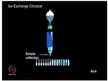
So analyze the contents these fractions for their protein content by using a UV-visible spectrophotometer at 280 nanometers.
