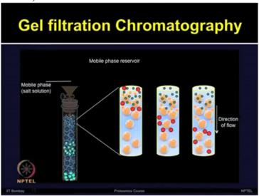
Now when protein sample is applied on to the column, the small proteins pass from the pores of the beads while the large proteins are excluded. Therefore this technique is also known as molecular exclusion chromatography.
