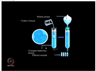
Mobile phase: The proteins are eluted of the column by using suitable mobile phase and then samples are collected by using different sample fractions.
