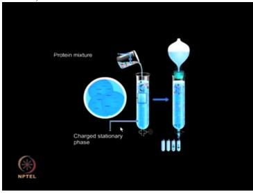
... and positively charged DEAE cellulose which is an anion exchanger
