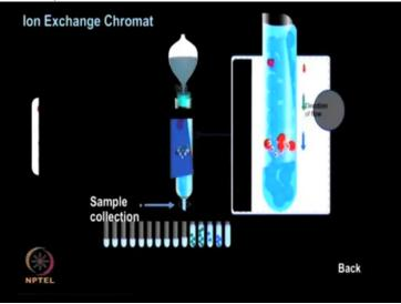
... will be present in the initial fractions while positively charged proteins that bound to the column are eluted in later fractions Once all the fractions are collected then the protein content can be analyzed by using spectrophotometer.
