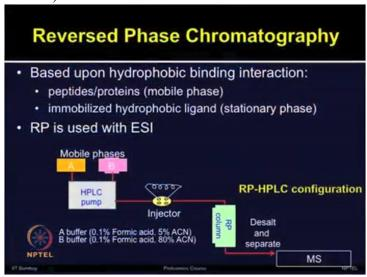
Molecules are bound on the column by means of hydrophobic interactions and are eluted out when the solvent polarity is modified.
