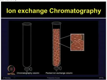
So in ion exchange chromatography, the column is packed with a resin, whether it is cation or anion exchanger depending upon the charge of the protein that need to be bound to the column and purified.
