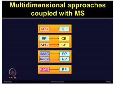
Now, third combination of using affinity chromatography as the first separation followed by Reversed Phase has been used. But what is most popular is the Strong cation exchange separation in first dimension followed by the Reversed phase chromatography in the second dimension.
