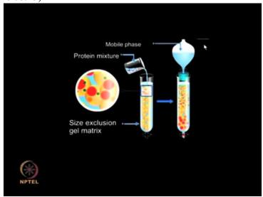
Mobile phase: the proteins are eluted out of the column by using a suitable mobile phase that carries the protein out for elution. For gel filtration a salt solution of appropriate strength is commonly used so that it will not have any effect on properties of proteins being purified.
