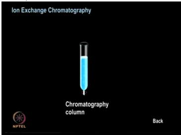
... the process in animation The column is packed with a suitable cation or anion exchange resin
