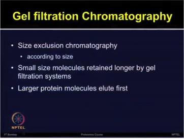
Gel filtration chromatography is also known as size exclusion chromatography. It means the molecules are separated according to the given size.
