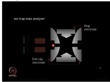
An ion trap makes use of a combination of ...
