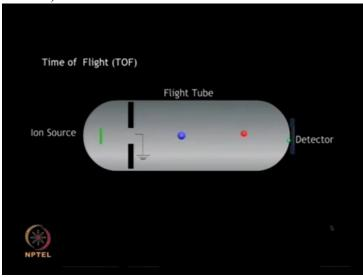
Ions are accelerated at different velocities depending on their mass to charge ratios.
