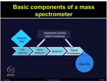
Sample inlet, it transfers the samples into the ionization source. The ion source or the ionization source, it converts neutral sample molecules into gas phase ions.
