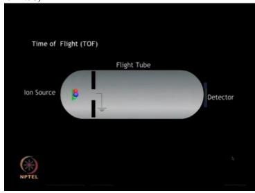
... MALDI along the long tube known as the Flight tube or TOF
