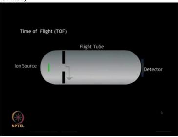
The Time Of Flight analyzer accelerates the charged ions generated by the ionization source...
