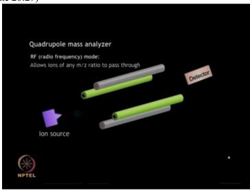
...in either radio frequency or scanning mode
