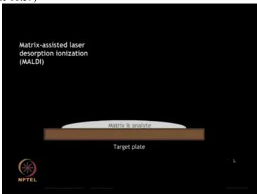
the analyte of interest is mixed with an aromatic matrix compound such as (Refer Slide Time 18:43)
