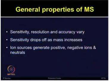
The sensitivity, resolution and accuracy vary among various mass spectrometers. The sensitivity drops off as the mass increases. And as I mentioned the sensitivity for protein detection can as low as atomolar or femtomolar range. Ion sources, they generate positive, negative and neutrals.
