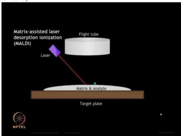
The evaporation of solvent leaves the analyte embedded in the matrix. The target plate is placed in a vacuum chamber with high voltage...
