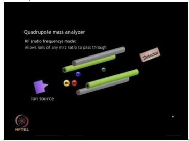
In RF mode or radio frequency ions of all m by z are allowed to pass through ...
