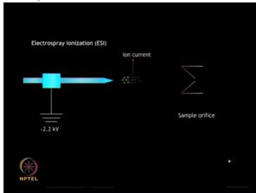
The droplets are formed in a very high electric field and become highly charged.
