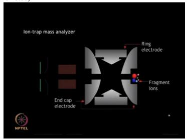
....using the electric field and measures the mass by selectively ejecting them to a detector.
