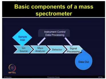
So although there are 3 major components involved; ionization source, mass analyzer and detector, but then there are some accessory components which are also equally important for doing the mass spectrometry based experiments.
