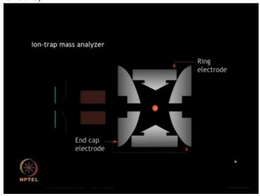
...electric and magnetic fields and captures ion in a region of vacuum system or tube Ion trap traps the ion ...
