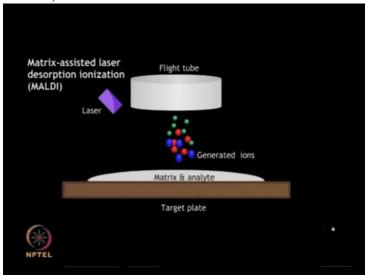
...gets absorbed by the matrix and is transferred to the analyte molecules...
