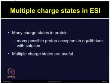
I will talk in more detail about how various types of ionization sources work that will be in the later part of the lecture. But just in this context I would like to mention that there are multiple charge states present in the ElectroSpray Ionization.
