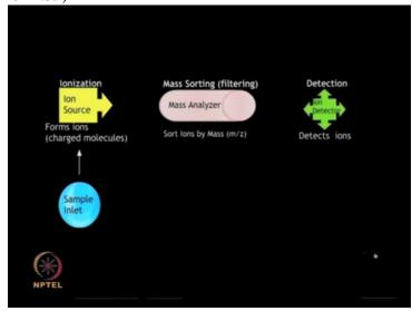
... by means of electric and magnetic fields ...
