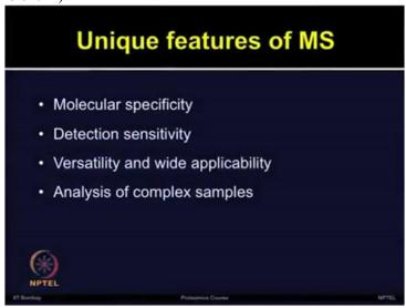
Molecular specificity, due to its unique ability to accurately measure molecular mass and provide fragment ions of analyte, mass spectrometry offers molecular specificity. It provides ultra high detection sensitivity. In theory MS can detect even a single molecule and its sensitivity at atomole and femtomole has also been demonstrated.
