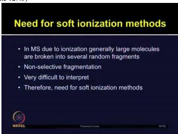
But these processes are too energy-rich to ionize intact large biomolecules and they lead to the unpredictable analyte decomposition. So for proteomic application, there was need for the soft ionization methods in mass spectrometry. (Refer Slide Time 13:05)
