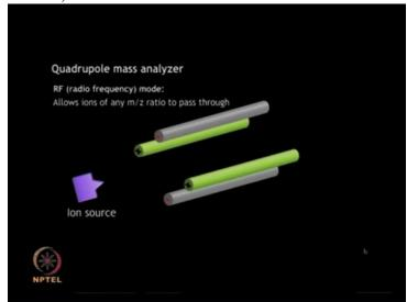
... to selectively stabilize or destabilize the paths of ion passing through a radio frequency RF quadrupole field. The Quadrupole mass analyzer can be operated ...
