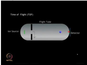
Ions of lower masses are accelerated to higher velocities and reach the detector first. The time of flight under such circumstances is inversely proportional to square root of molecular mass of the ion. The TOF analyzer ...
