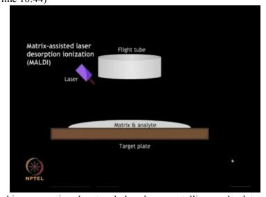
This is dissolved in an organic solvent and placed on a metallic sample plate.
