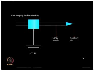
....from the tip of a fine metal capillary....
