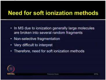
These are non-selective fragmentation. The hard ionization is very difficult to predict. So, therefore it led to the need for soft ionization methods in proteomics. What are different properties of ionization sources?
