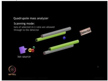
...will move towards the detector and the rest can be filtered out.
