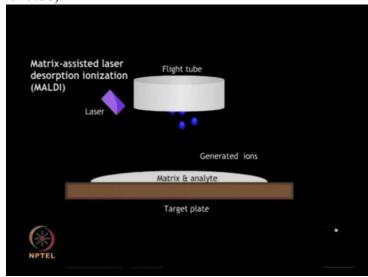
These ions then accelerate towards the mass analyzer based on their mass-to-charge ratio.
