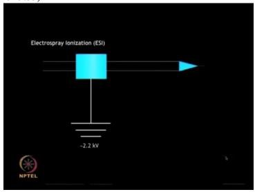
In ElectroSpray Ionization, the sample is present in the liquid form and ions are created by
