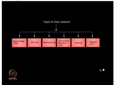
Currently various types of mass analyzers are available including Time Of Flight, Ion Traps, Quadrupole, Ion Cyclotron Resonance, Orbitrap and Magnetic Sector.
