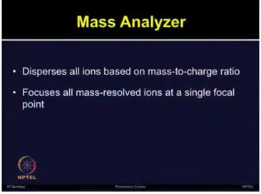
First of all it disperses all the ions based on their mass to charge or m by z ratio. Secondly, it focuses all the mass-resolved ions at the major, single focal point. So therefore all the ions enter in mass spectrometer, it can maximize their transmission.
