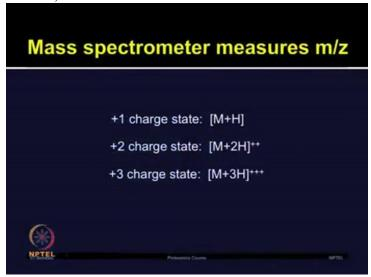
So the mass spectrometer measures m by z. The MS data is presented as mass to charge ratio, which is mass of an ion "m" divided by the number of charges "z" it carries. So, the total charge on ion is represented by q equals to "z""e", where e is the charge on an electron
