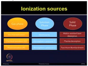
With the gas phase, electron ionization, chemical ionization and photo ionization, these are the commonly used ionization sources.
