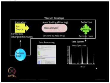
It is being increasingly used for detection and analysis of proteins from the complex samples. The various components which are involved in the mass spectrometry experiments are shown here
