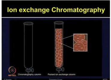
So in ion exchange chromatography, the column is packed with a resin whether it is cation or anion exchanger depending upon the charge of the protein that needs to be bound to the column and purified.
