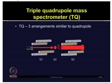
Now triple quads, which is arrangement of quadrupoles is widely used for the proteomics. In triple quad, Q1 it casts the ionic streams. It directs ions of a selected m by z ratio into the second quadrupole, Q2 which is a collision cell.
