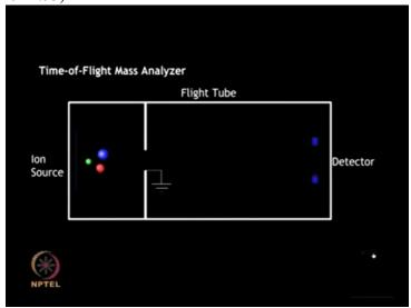
or the reflectron mode which depends on the sample to be analyzed. In case of small molecules this mode usually provides sufficient resolution.
