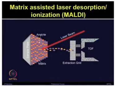
The ionization source is responsible for converting analyte molecules into gas phase ions in vacuum. This has been made possible by the development of soft ionization techniques...
