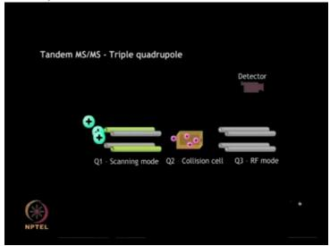
ions enter the collision cell where they are fragmented by collision against an inert gas like argon.
