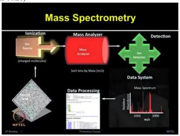
Mass spectrometry is technique for protein identification and analysis by production of charged molecular species in vacuum and its separation by magnetic and electric fields based on mass to charge ratio.
