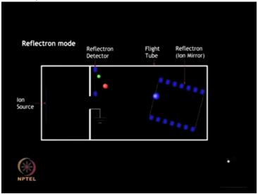
So, rather than using very long time of flight tubes; by including the reflectron ion mirrors, we can increase the path length. This helps to even out any kinetic energy differences between ions having the same mass and thereby improving the resolution.
