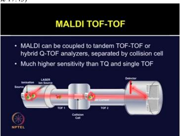
MALDI TOF-TOF; that is one of the widely used tandem-MS configuration. In this one the TOF-TOF or two time-of-flight tubes as well hybrid quadrupole time-of-flight analyzers can be used.
