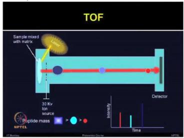
In time of flight tube, the ions are accelerated to high kinetic energy, and due to different velocities, they are separated in a flight tube. As I mentioned earlier, by adding the reflectron or a reflector, the ions can turn around in the reflector that can compensate for minor differences in the kinetic energy.
