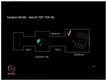
and further resolved on the basis of their m by z values in the second Time Of Flight tube, after which they can be detected.
