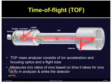
So the TOF mass analyzers, they consist of ion acceleration and focusing optics and a flight tube.
