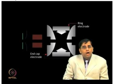
The Ion Trap, it traps ions using electrical fields ...
