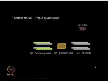
The triple quadrupole consists of two sets of parallel metallic rods interspersed by a collision cell. The first quadrupole scans the ions coming from the ionization source and allows only ions of a particular m by z ratio to pass through.
