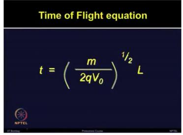
The Time of Flight of a charged ion can be calculated by using the equation shown in this slide, the flight time is directly proportional to the square root of mass of the ion.
