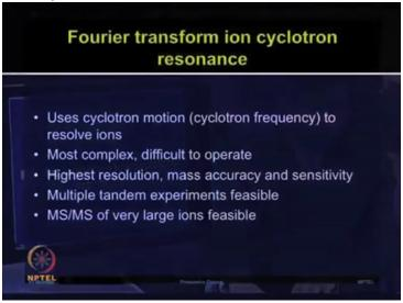
An FT-ICR MS can be considered as ion trap system where ions are trapped in the magnetic field. It uses cyclotron motion or cyclotron frequency to resolve the ions.
