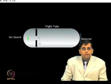
The Time of flight measures the m by z ratio
