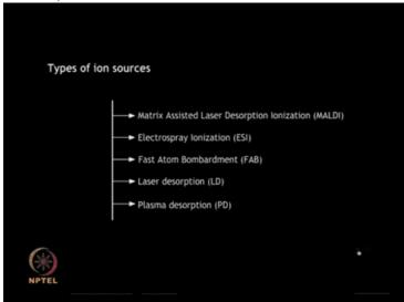
Additionally there are other ionization sources such as Fast Atom Bombardment FAB, Laser Desorption LD, Plasma Desorption PD. We discussed the two most commonly used soft ionization techniques MALDI and ESI.
