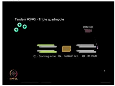
based on the varying behavior of ions in an oscillating electrical field.
