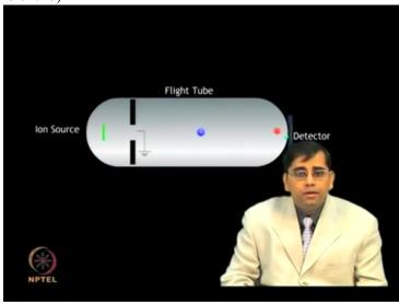
...the time it takes for ions to fly in the analyzer and strike to the detector.
