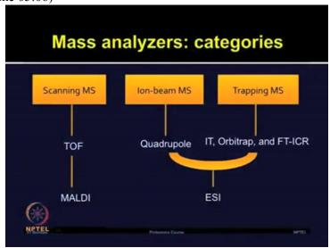
Now mass analyzers can be categorized broadly into the scanning MS, ion-beam MS and trapping MS. Scanning MS is more commonly used with TOF which is further coupled with the MALDI ionization sources.
