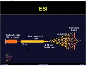
... which ensures that the non-volatile protein sample is ionized without completely fragmenting it Most commonly used ionization sources are MALDI and ESI.
