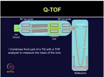
Q-TOF. The Q-TOF, it combines front part with quadrupole or it can be triple quad TQ along with the TOF analyzers to measure the mass of ion.
