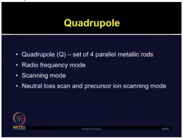
So, as we talked, quadrapole is set of 4 parallel metallic rods with opposite pairs are electrically connected.
