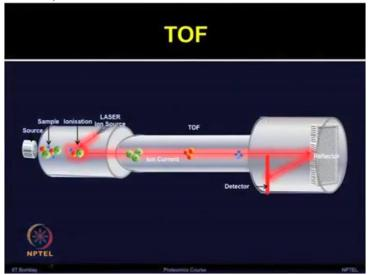
In TOF, the ions are accelerated to high kinetic energy and due to their different velocities; they are separated in a flight tube. One can also use the reflectron mirror so that ions can turn around into a reflector and it compensate for minor differences in the kinetic energy and provide long separation.
