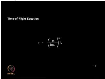
The time of flight of a charged ion can be calculated by means of the equation shown here. The flight time is directly proportional to the square root of mass of the ion.
