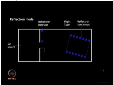
A reflectron which acts as a ion mirror is incorporated at one end of the time of flight tube.
