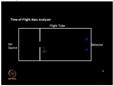
the ionization source, on the basis of their mass to charge ratio. The time of flight tube can be operated in the linear mode ....
