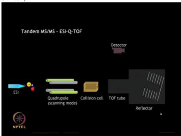
ESI-Q-TOF is another common tandem MS configuration that first selects ions in the radio frequency mode.
