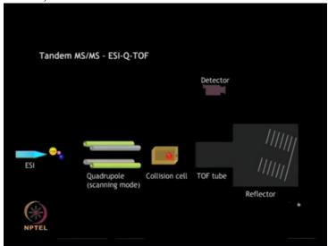
Selected peptides are fragmented in collision cells and resulting ions are accelerated and resolved on the basis of their time of flight.
