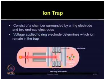
It consists of a chamber which is surrounded by a ring electrode and two end-cap electrodes, as you can see in the figure here. The voltage applied to the ring electrode determines which ions remain inside the trap. So ions above a threshold of m by z ratio, they remain inside the trap and others can be ejected through a small hole.
