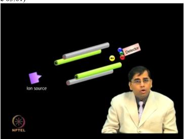
oscillating electric field that is created by applying direct current and radio frequency potentials to these electrodes
