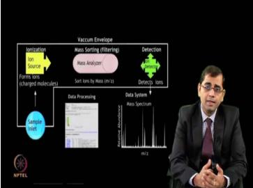
Mass spec is highly sensitive, balanced to measure the mass of the molecule in vacuum based of mass to charge ratio. It consists of an ionization source to ionize the molecule, a mass analyzer resolve the analyzed molecules in vacuum, and detector to read the signals coming from mass analyzer.
