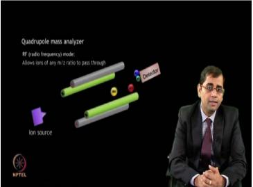
... Time of Flight TOF, Quadrupoles and Ion Traps
