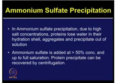
So let's talk about ammonium sulfate precipitation which is one of the most previously used methods for the classical way of performing the experiments. The ammonium sulfate precipitation was used, although its use is not so common when you are preparing samples for the proteomic application but this one still remains a good choice.
