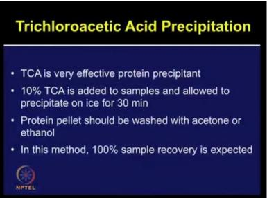
Now let's talk about TCA or trichloro acetic acid precipitation. TCA is one of the very effective protein precipitant. One can use 10 to 20% of TCA, usually 10% TCA is commonly added to the samples and then allowed to precipitate in the ice condition for almost half an hour to one hour.
