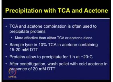
So this is very easy method to precipitate out the protein. First add 10% TCA with acetine and after centrifugation, wash the pellet to remove the TCA which could be present there and then further wash 3 or 4 times with acetone containing DTT. After that you need to dry out your pellet so that any residual amount of acetone is not remaining in pellet
