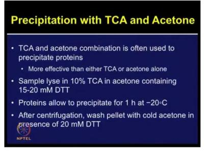
So this combination has demonstrated that it can precipitate the proteins more efficiently which could not be achieved either by using TCA alone or by using acetone alone. So a recommended concentration, one can try; lyse samples in 10% TCA made in acetone, and also add 15-20 milli molar of DTT.
