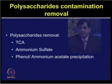
During the precipitation step itself, lots of polysaccharides, they get removed. So TCA, TriChloro Acetic acid, ammonium sulfate or phenol or ammonium acetate precipitation, they are efficient ways of removing the polysaccharide contamination.
