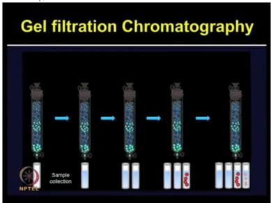
After these steps, the fractions are collected and analyzed for the protein content. So you can expect that larger proteins shall elute first, and then the small molecules will be eluted later. So gel filtration chromatography is useful for removal of even contaminants, doing desalting steps as well as for buffer exchange. However its drawbacks are its low capacity, broad distribution of pore size and small sample volumes to be analyzed.
