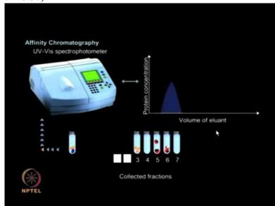
The fractions are then analyzed for their protein content using a UV visible spectrophotometer at 280 nanometers.
