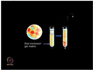
Let's first give the definition of few components. Size exclusion gel matrix, the matrix filling the gel filtration column consists of a highly hydrated polymeric material commonly dextran, agarose or polyacrylamide.
