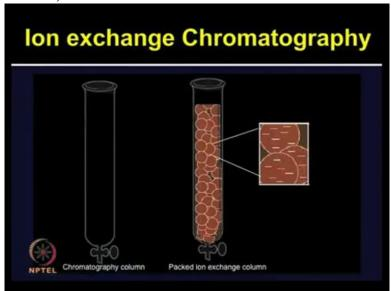
So ion exchange chromatography, the column is packed with the resin, whether it is cat-ion or an-ion exchanger depending upon the charge of the protein that needs to be bound to the column and purified.
