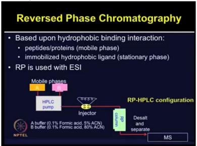
Let's first talk about Reversed phase RP Chromatography. The Reversed-phase chromatography is based upon the hydrophobic binding interaction between the peptides or proteins in the mobile phase and immobilized hydrophobic ligands in the stationary phase.
