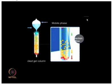
The column is then eluted with a salt solution of appropriate concentration.
