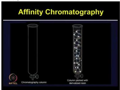
So in affinity chromatography, the column is packed with resin which is covalently coupled to the ligand specific to the protein of interest. The protein mixture is passed over the derivatized affinity column.
