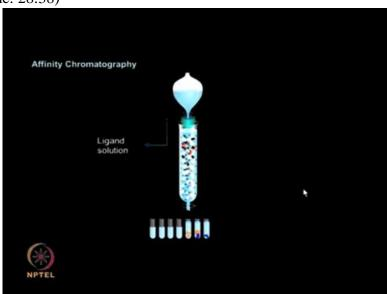
After the column has been washed thoroughly, the protein of interest is eluted by passing a ligand solution which binds to the matrix-bound protein and removes it from the column.
