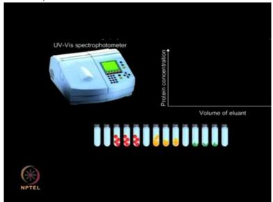
Now analyze the protein content by using UV visible spectrophotometer at 280 nanometers.
