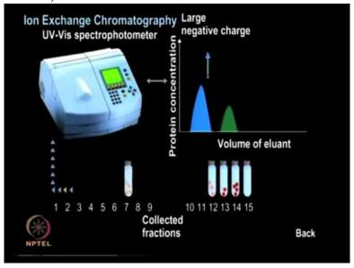
In this particular example, the negatively charged large molecules coming first and then positively charged fractions are coming later.
