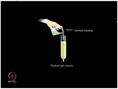
This packed gel matrix is then loaded with the protein sample containing mixture of unpurified proteins of different sizes.
