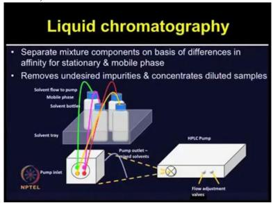
So what is Liquid Chromatography? The Liquid Chromatography separates mixture components on the basis of differences in the affinity of stationary and mobile phase. It can remove the undesired impurities.
