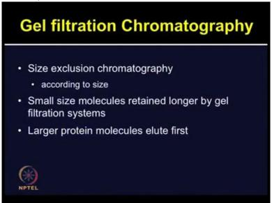
So gel filtration chromatography is also known as size exclusion chromatography. It means the molecules are separated according to the given size. The small molecules, or even if you are separating small molecules such as salt, those will be retained longer by the gel filtration system and larger molecules such as proteins will elute first because they cannot enter inside the porous...these beads and they can be used to separate proteins based on the size.
