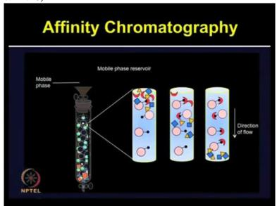
Now the column is washed with a suitable mobile phase to remove the unbound protein and protein of interest which has higher affinity for the ligand remains bound to the derivatized column matrix and is not removed during the washing step.
