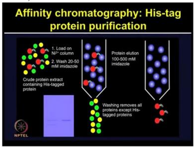
Now after washing with the mild imidazole such as 20 to 50 milli-molar, unbound residues will come out but by increasing the concentration such as 100 to 500 milli-molar of imidazole, the proteins can be eluted out.
