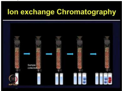
So if you have negatively charged protein which gets eluted first will be present in the initial fractions while the positively charged protein that bound to the column will be eluted in the later fraction or it will be vice versa.
