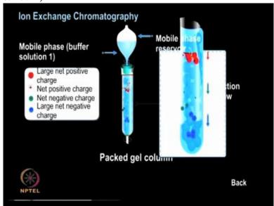
The column is eluted with a buffer solution of suitable pH such that the negatively charged molecules are removed from the column while the positively charged molecules remain bound to the anion exchange resin.
