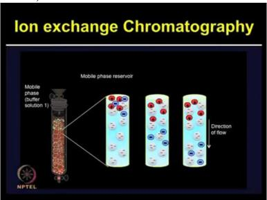
So proteins are adsorbed to the ion exchange column and then it can be de-adsorbed by increasing the salt or altering the pH of the buffer which can change the charge on protein. So various anionic buffers such as acetate and phosphate are used for cat-ion exchange and cationic buffers such as Tris chloride or ethanolamine are used for the anion exchange.
