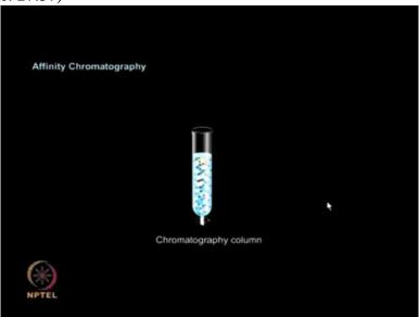
Now let's see the process in the following animation. The column is first packed with a suitable resin that has been covalently coupled to the ligand specific to the protein of interest.
