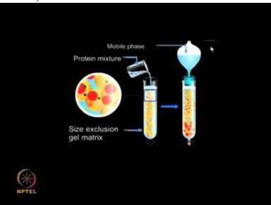
The protein mixture is a mixture of unpurified proteins of different sizes which is applied on the top of the column.
