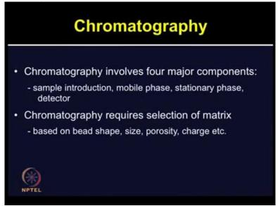
The chromatographic technique involves 4 major components; an inlet for sample introduction, the mobile phase, stationary phase and a detector. Each type of chromatography requires very educated and informed choice of matrix considering the bead shape, size and porosity. In addition to the functional group type, the charge, distribution and density as well as elution conditions such as the pH, the ionic strength and gradient shape.
