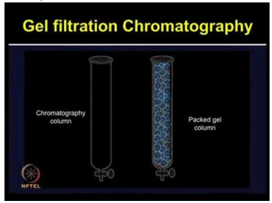
The gel filtration column is composed of porous beads which are made from polyacrylamide, dextran or agarose. Now these columns are packed with hydrated porous gel matrix.
