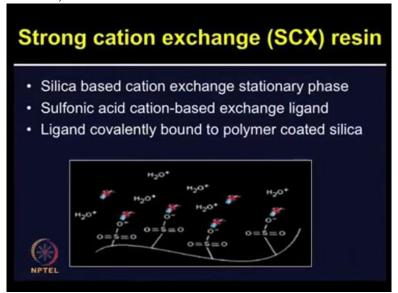
Let's now talk about strong cat-ion exchange or SCX chromatography. SCX consists of a stationary phase matrix which is made up of negatively charged sulfonic acid groups which bind the oppositely charged peptide molecules. These molecules can be eluted out using a positively charged mobile phase which binds the analyte molecules more firmly.
