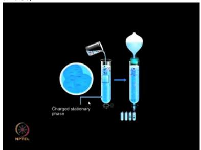
The charge in stationary phase, the column in stationary phase consists of a positively charged or negatively charged polymeric matrix which will bind molecules of the opposite charge. Commonly used ion exchangers include negatively charged Carboxy Methyl cellulose or CM cellulose which is a cation exchanger and positively charged DEAE cellulose which is anion exchanger.
