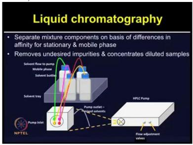
It is mostly used for separating the peptide mixture. One of the diagrams is shown here; which is a typical Liquid Chromatography setup which consists of solvent bottles,
