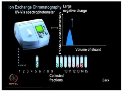
Analyze the contents, these fractions for their protein content by using a UV visible spectrophotometer .at 280 nanometers. A graph of eluent volume versus protein concentration can then be plotted.
