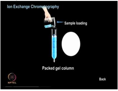
The an-ion exchange column is then loaded with the impure protein mixture consisting of various positively and negatively charged proteins.
