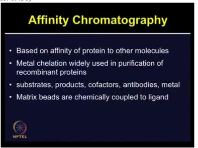
So affinity chromatography is based on affinity of proteins to its ligands or other molecules. The metal chelation is widely used in purification of recombinant proteins where substrates, products, cofactors, antibodies or metals, these can show affinity for given protein and this is used for strategy to purify the proteins based on its affinity. The matrix beads are chemically coupled to these ligands.
