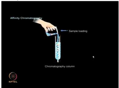
This derivatized affinity column is then loaded with the protein mixture containing various proteins having different properties and interaction specificity.
