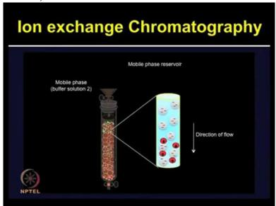
Now the buffer solution is changed so that the net pH of the protein of interest can be modified and it no longer binds to the ion exchange resin.
