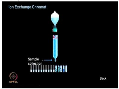
Therefore the bound protein also gets eluted out of the column in this manner. The fraction of appropriate size must be collected and analyzed for their protein contents. The negatively charged proteins which get eluted first will be present in the initial fractions...
