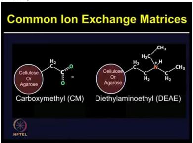
So in this slide, some of the common ion exchange matrices are shown like CarboxyMethyl CM, and DiEthyl AminoEthyl DEAE. So when a desired protein is positively charged, the cat-ion chromatography should be used, when a desired protein is negatively charged, the anion exchange chromatography method should be used.
