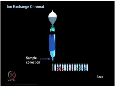
... while positively charged proteins that bound to the column are eluted in later fractions. Once all the fractions are collected then the protein content can be analyzed by using a spectrophotometer.
