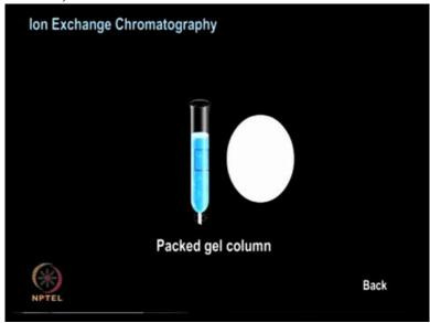
After giving you brief description of the components let me show you the process in animation. The column is packed with the suitable cation or anion exchange resin depending upon the charge of the protein that needs to be bound to the column and purified.
