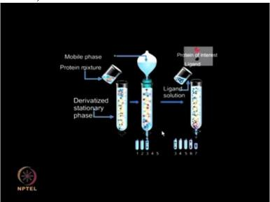
The ligand solution: The solution is passed through the column to elute the bound protein of interest since it contains the same ligand that is bound to the column matrix. It is capable of eluting the proteins by interacting with it.
