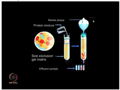
Mobile phase, the proteins are eluted out of the column by using a suitable mobile phase that carries the protein out for elution. For gel filtration, a salt solution of appropriate strength is commonly used so that it will not have any effect on properties on the proteins being purified.
