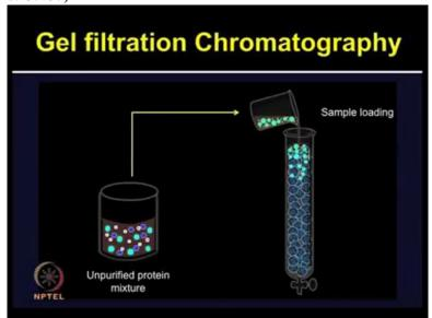
The protein sample which contains a mixture of unpurified proteins of different size is then loaded on these columns.
