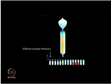
The largest proteins eluting out first will be present in the initial fractions while the smaller fractions which elute out later will be present in the later fractions. Once all these fractions are collected, then it can be analyzed for their protein content by using a UV visible spectrophotometer.
