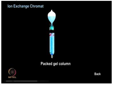
The buffer solution is changed such that net pH of the protein of interest is modified and no longer binds the ion exchange resin.
