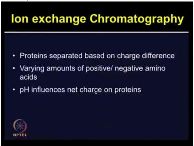
In ion exchange chromatography, the proteins are separated based on charge difference. The proteins with overall negative charge will interact with positive charges or the vice versa. So by varying the amount of positive and negative amino acids and even pH can influence the net charge on proteins.
