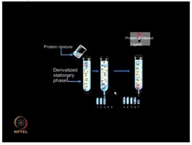
The protein mixture: It is unpurified protein mixture which consists of proteins having different properties and interaction specificity for the ligand bound to the column matrix.
