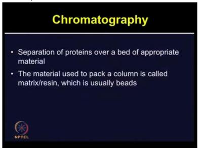
So let's talk about what is chromatography? So, chromatographic methods involve separation of proteins over a bed of appropriate materials. These materials are usually packed in a given column and known as matrix or resin. So these matrix and resins, they are usually beads with or without attached chemical groups. Now the binding and interactions of proteins with the column matrix is an important feature of chromatography.
