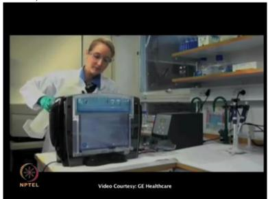
fill the top compartment with cathodic running buffer. Program the power supply according to recommendations and run second dimension. Protect it from light for approximately 4 to 5 hours or until the dye front reaches the bottom of the gel.
