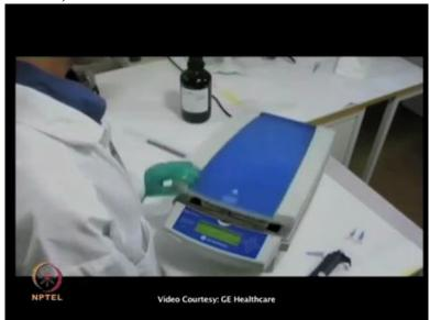
The lid is closed to protect the fluorescent samples from light. The instrument was programmed according to recommendation and run overnight.
