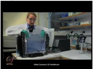
In the second dimension SDS PAGE the proteins will be separated according to molecular weight and this is performed with Ettan DALTsix system.
