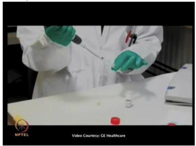
The first step in 2D electrophoresis is to prepare IPG strips for rehydration.
