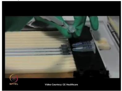
50 micrograms from each sample were applied using sample application caps.
