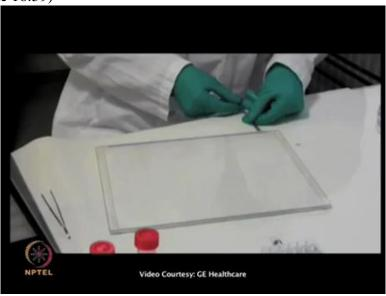
Avoid trapping air between the strips and the gel.
