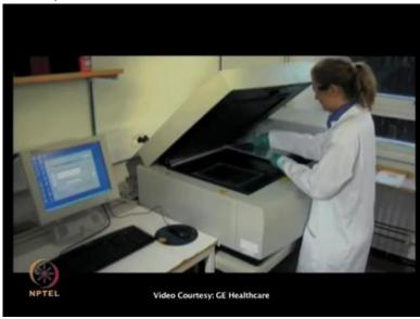
After the second dimension electrophoresis, the gel cassettes are placed by using the grippers in the Typhoon FLA gel imager.
