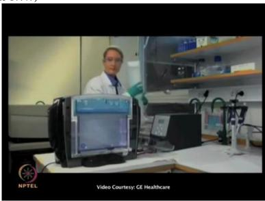
Fill the electrophoresis chamber with anodic running buffer. Insert the gels and
