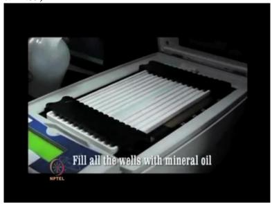
Fill all the adjacent wells with mineral oil to ensure uniform current flow.
