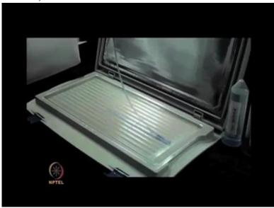
IPG strips are used for separation of proteins based on their Isoelectric Point.
