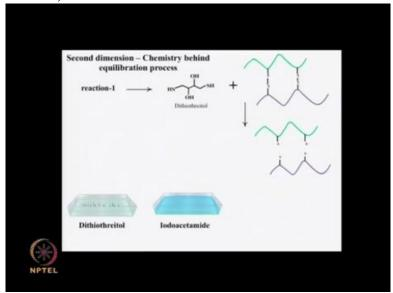
The dithiothreitol enables cleavage of all disulfide bonds present in the proteins in the IPG strip.
