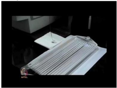
Carefully remove the IPG strip from the rehydration tray and drain out any excess oil by blotting it on a tissue paper.
