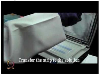
. Transfer the IPG strip into this solution after draining off any excess liquid from the first.
