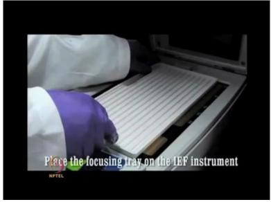
Place the focusing tray on the instrument and...
