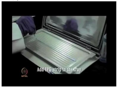
These are Acrylamide coated plastic strips containing immobilization of various pH spread across it. They have successfully replaced conventional tube gels due to their reproducibility they can achieve.
