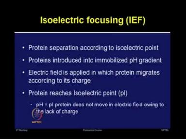
You can take the Immobilized pH Gradient Strip and apply the protein solution on the IPG strip so that protein is absorbed on this strip. And then after applying the electric field, the proteins will migrate according to its charge.
