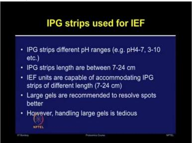
Now these IEF units or Isoelectric Focusing Units obtained from different vendors, commercial manufacturers, they are capable of taking the IPG strips of different varying pH length.
