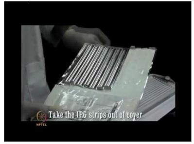
Then remove the IPG Strip from its cover and place it carefully in the well.
