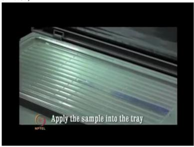
Clean all the apparatus thoroughly before use to avoid any contamination. Add the reconstituted protein sample in a well of the rehydration tray.
