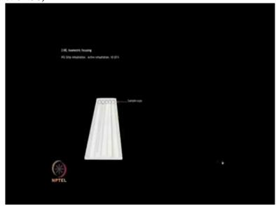
... where the protein sample is added to the strip via a sample cup...
