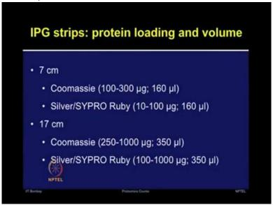
These are some recommendations for how much proteins one should load on the IPG strips. For example, if you have small strip like 7 centimeter length, you can apply between 100 to 300 microgram of protein and maximum volume could be 150 to 160 micro liters. Usually Coomassie stain is a good choice and if you have Coomassie stain, you can stain that with this much protein.
