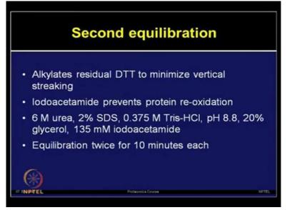
Now this buffer recipe is also exactly similar to the last one except one change, DTT is replaced with iodoacetamide. So you can add 135milli molar of iodoacetamide during the second equilibration step. Now this is very important because IAA can alkyl ate the residual DTT and it minimizes the vertical streaking. It also prevents the re-oxidation.
