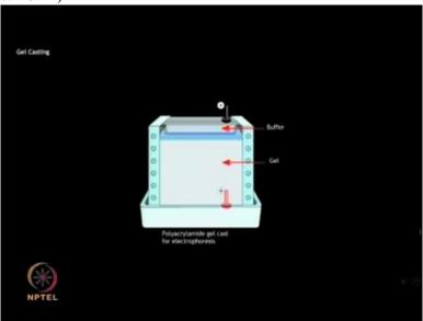
The molecular dimensions of the pores can be controlled by varying the amount of n n'-methylenebisacrylamide. Once the solution is poured, then the sample wells can be created.
