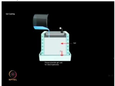
Ammonium persulfate and TEMED are added to facilitate the generation of free radicals and cross-linking.
