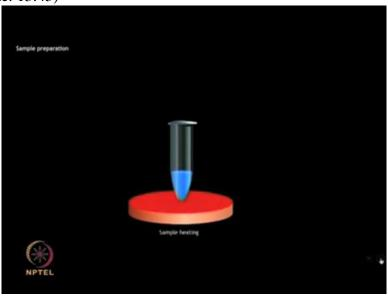
The DTT used breaks any disulfide linkages that may be present during the process you boil or heat your protein samples...
