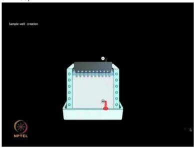
... which is placed in the gel, as soon as it has been poured.
