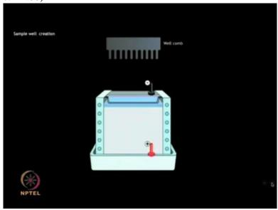
The sample wells of uniform size, shape and separation are made using a comb....
