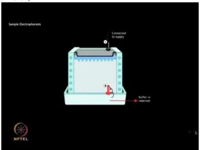
A direct current supply between 100 to 350 Volts is passed depending upon the size of gel...
