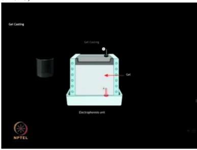
The gel is prepared by free radical induced polymerization of acrylamide and bis-acrylamide in a suitable buffer.
