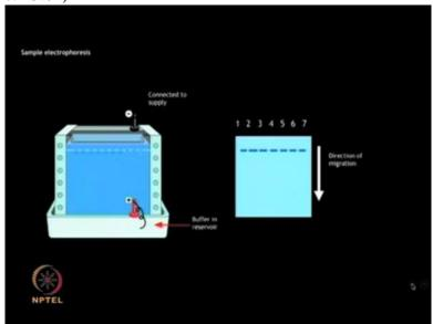
... to separate the protein mixture into discrete bands based on their mass, charge to mass ratio.
