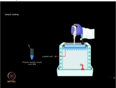
The protein samples can be loaded on the wells by using a micropipette. As you can see in the animation you can use different wells to load different types of samples. Once all the samples are loaded, then you can take this unit and move into electrophoretic apparatus.
