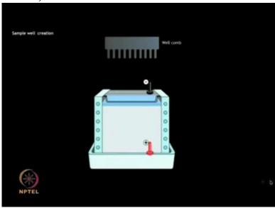
The sample wells of uniform size, shape and separation are made using a comb...
