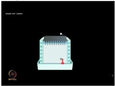
... which is placed in the gel as soon as it has been poured
