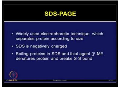
So SDS PAGE is one of the very widely used electrophoretic techniques which separate protein based on their size or their molecular weight. So this molecule SDS or Sodium Dodecyl Sulfate which is an anionic detergent, it provides negative charge. It binds at a ratio of 1.4 gram of SDS per gram of protein to provide almost similar charge to mass ratio.
