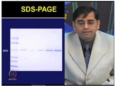
I am showing you one SDS PAGE image in which, from the left to the right, you can see; the first lane is the standard or the known molecular weight. In this well you can see there are different, at least 5 or 6 bands are visible. These are the known molecular weights, sometimes starting from 150 kilodalton to 10 kilodalton of molecular weight range.
