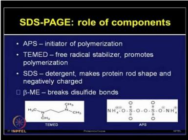
TEMED, that is a free radical stabilizer. It also promotes the polymerization of the gel process. So beta Mercaptoethanol is not used in making the gel, but for your protein treatment to break the disulfide bond.
