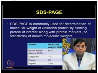
So SDS PAGE is one of the very commonly used methods for determining the molecular weight of protein of your choice or unknown protein which you want to know how much molecular weight it is.
