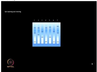
The larger proteins are retarded in the gel and remain close to the point of application while the smaller proteins migrate further along the gel. The gel can then be stained with Coomassie brilliant blue and viewed to observe various discrete protein bands.
