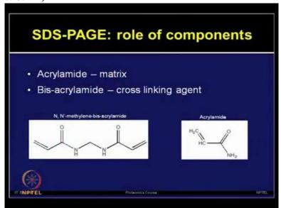
Acrylamide, it provides the matrix or gelling for making the gels. Now Bis-acrylamide, that is a cross-linking agent. By adding both Acrylamide and Bis-acrylamide in a fixed ratio, one can make the gel by adding the gelling agent and the cross-linking agent.
