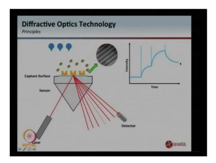
So, the sensors surface is a piece of glass it has lines as you can see in this inset and when I shine light through it this going to be a very faint signal. Now, suppose I introduce molecules that bind on this line the signal gets darker and it is represented in the hand side here by the intensity of lights. So, effectively if I have a detector in one location you can see that the signal increases with time as binding takes place.
