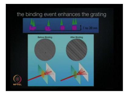
That is right. So, again let me just show you different vision or we have here the grating made up of individual protein molecules, and then binding takes place on it more binding takes place and what happens is here is this surface is before binding, and you can see that if the coverage is not very strong after binding the coverage is strong, and you get much a bigger signal intensity of signal. That is right.
