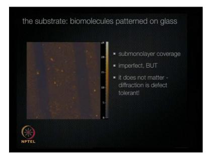
This protein on the piece of glass and it is sub monolayer coverage. It is very small various parts amount of protein in there, and it is imperfect as you can see not even at all but it is does not matter, because diffraction is defect tolerant. What do you mean by defect tolerant? Because, if there is some defect are we going to have different type of diffraction pattern or that can be compensated because of the nature of diffraction.
