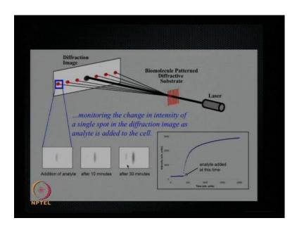
That is right. So, in our assessor in our first implementation it is diode laser a laser pointer and a webcam in these are actually pictures captured from webcam. So, actually monitor the change in intensity in one spot of the diffraction image up an addition of analyte. So, after few minutes its gets darker and then gets darker even there.
