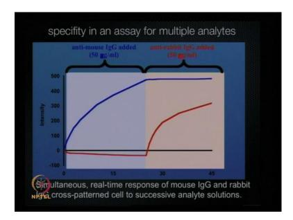
This is mouse IgG on one analyte; the other one is rabbit IgG so, when we introduce anti mouse IgG you can see the increasing signal in one of the spots, but not in the other spot. The red versus, the blue, and then at this point we introduce anti rabbit IgG in which case one of this spots the second spot increase, but the first one just remain constant.
