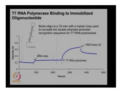
So in this case, as long as we are reasonably at the certain range of concentration the intensity is linear with concentration and therefore, you can actually model the kinetics nicely. It is just a, this is the similar experiment and this is under binding of polymerase RNA polymerase to their immobilized oligo.
