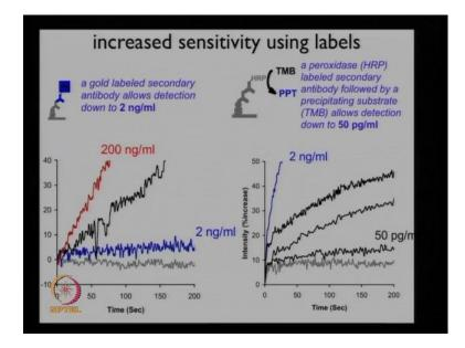
So, you remember that we have the 200 nanograms per ml that I was in the previous slide. But now I am going to introduce a secondary, here is a secondary antibody and in this case a label with a little piece of gold actually, we found a later we do not need that gold label. But anyway for this graph, that was had a gold label in there and we can bring it down 200 nanogram per ml to 2 nanograms per ml. That is fine.
