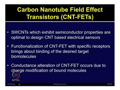
The successful combination of carbon nanotubes with filed effect transistors has led to the development of this novel sensing device known as Carbon nanotube field effect transistor. As we have discussed the different type of carbon nanotubes, single walled SWCNT's and multiple walled MWCNT's the SWCNT's or single walled carbon nanotubes, which exhibit semiconductor properties are optimal to design the carbon
