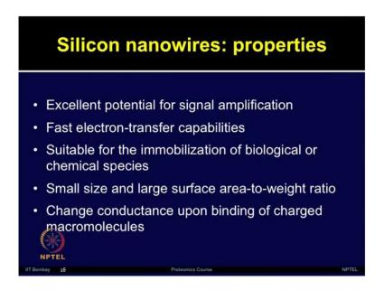
Let us discuss some of the properties of Silicon nanowires they have very high potential for signal amplification they have Fast electron transfer capability silicon nanowires are Suitable for the immobilization of various biological and chemical species. They are Small size and have large surface area to weight ratio. Again the Change in the conductance is measured here upon binding of charged macromolecules.
