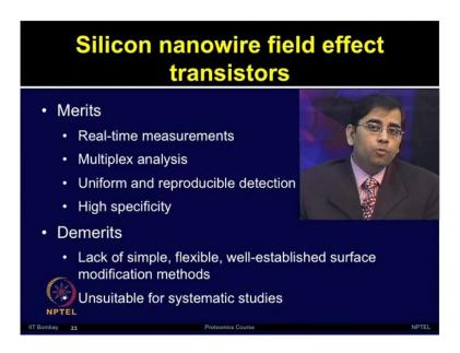
So, continuing on to the Silicon nanowire field effect transistors their different Merits and Demerits. So, this platform provides us the real time measurement capability also it offers multiplexing analysis, that is uniform and provides reproducible results for various biomolecular detection and it shows very high specificity. Now discussing about
