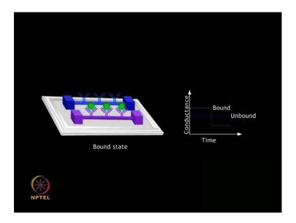
So, that we can understand the principles more clearly. Silicon nanowire field effect transistors silicon nanowires can be functionalized with several chemical and biological species and used as sensitive detection devices antibodies are commonly immobilized on silicon nanowires for detection of protein antigens.
