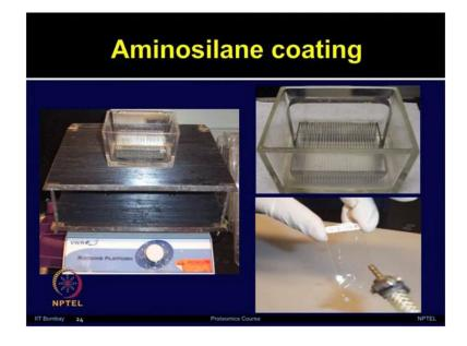
At the bottom panels of the right side, I have shown that these slides, can be either centrifuged or dried with the compressed air and then those are ready for further printing purpose.
