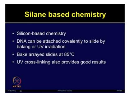
So, let us focus more on the Silane based chemistry. We want to talk about printing the DNA on the chip surface, for using cell free expression based NAPPA protein microarrays. So, silicon based chemicals, they contain two types of group the inorganic groups such as, alkoxy groups like methoxy or ethoxy or oregano functional groups such as, amino epoxy viral etcetera.
