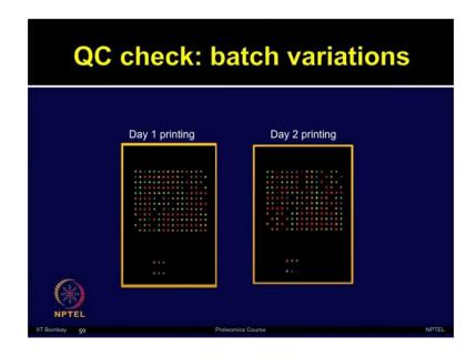
And, if you print the GST protein in the dilution series as shown side, which is printed in the bottom of the slide, those can be used for assessing how much protein is produce on each feature, so batch to batch c v, sample to sample coefficient of variation as well as replicate coefficient of variations should be calculated.
