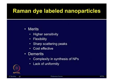
Which includes high sensitivity, the flexibility due to the non overlapping probes very sharp scattering peaks, as well as the cost effectiveness of the assay. However, there are certain demerits of using Raman dye labeled Nanoparticles which includes the complexity in synthesis of these Nanoparticles, as well as the lack of uniformity.
