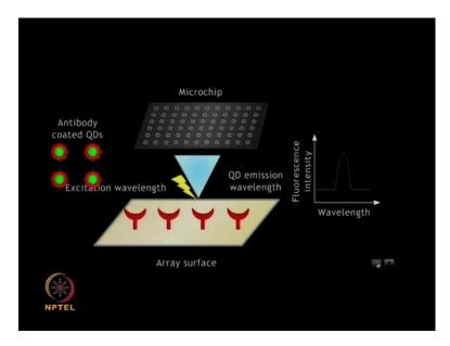
Let us now look at this animation for the quantum dots, to understand it is functioning in a better way. Changes in the emission wave length upon binding to the antibody conjugated quantum dots are recorded by the micro chip and use for detection of various biomolecules. Quantum dots are capable of detecting molecules down to femto molar levels and provide significant advantages, over conventionally used organic fluorophores. In this interaction we will see how quantum dots work.
