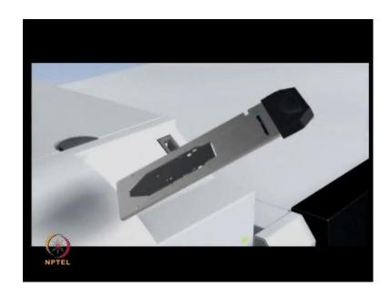
The Agilent HPLC chip, integrates enrichment and analytical columns, microvalve connections and metal coated nanoelectrospray tip on an inert multilayer polymer film, and it is smaller than a credit card. The compact architecture of the Agilent HPLC chip reduces peak dispersion, and combines all steps from sample loading through compound ionization for seedless operation.
