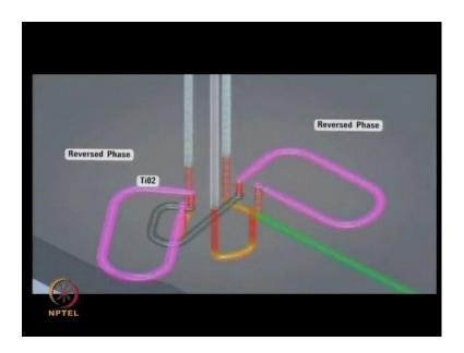
Moving beyond protein identification, the new phosphor chip with sandwiched reversed phase titanium dioxide trapping column; provides researches working on post-translation modification with a convenient tool targeted at phosphorylated peptides.
