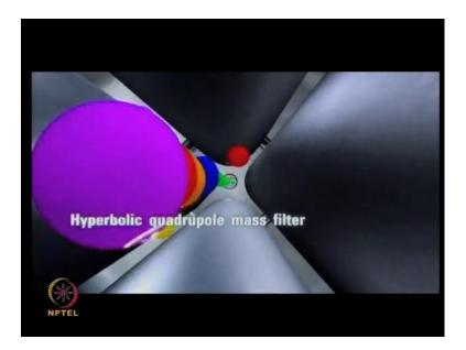
The first quadrupole mass filter allows only ions of the target mass to pass through, the hyperbolic shape of the rods enhances ion transmission and spectral resolution.
