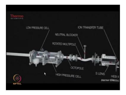
If you look at the schematic of the system and the front part of the system, it is the ionization source which sits on the front. Then you have the transfer optics, and the transfer optics we have the s lens which is the newest generations transfer optics, and
