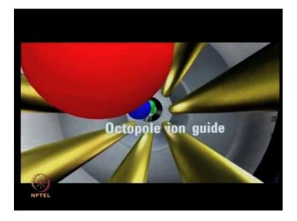
And on access octopole ion guide provides nearly one hundred percent ion transmission over a wider mass range. Having the lenses enhance high mass ion transmission and increase sensitivity over a wider mass range.
