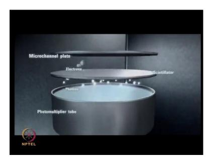
The microchannel plate detector converts the ions signal from the electrons to photons and back to electrons. This electrically isolates the high voltage flight tube and front of the detector from a signal pass to the electronics;
