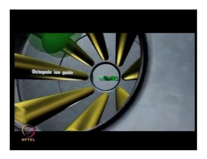
Another Octopole ion guide keeps the ions together while allowing excess collision gas to be pumped away, a quadrupole ion guide flattens the stream of ions for better transmission through the slicer;
