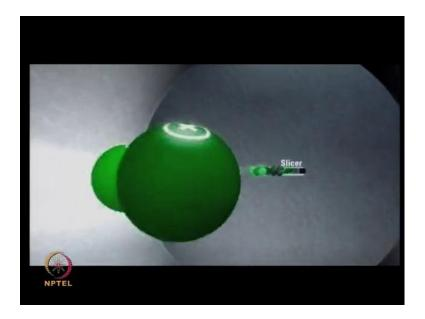
The slicer reduces variations in the vertical momentum of the ions. Ions with too much vertical momentum do not reach pulser; this improves mass accuracy for all ions. The flight tube is constructed a special materials with very low collision of the thermal expansion, so it is less sensitive to temperature changes.
