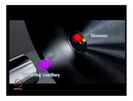
A thin skimmer aperture, carefully matched, whole size and short capillary to skimmer distance reduce being broadening.
