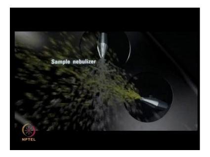
A second nebulizer, introduces reference mass solution that ensures continue mass access correction to the best possible mass accuracy, high-volume counter-flow drying gas reduces noise related to incomplete drying solvent droplets, and keeps the sampling capillary and ion optics cleaner for reduce maintenance.
