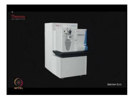
Just introducing the newest technology that is LTQ orbitrap elite, in the LTQ orbitrap elite if you look at this hybrid systems which has two mass spectrometer, the mass spectrometer which is sitting front as a linear trap, so LTQ orbitrap velos, and then the back and which is there is the high field orbitrap or called the orbitrap elite.
