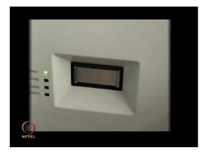
So, click on the software and open the acquisition window and then click on the open door, insert MALDI target plate face up with the cut-off corner to the front and
