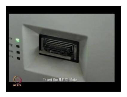
Now by using software close door. The door of insertion chamber is now closed you can select the plate; you can view the overall plate on the screen and then select a spot which you want to analyze.
