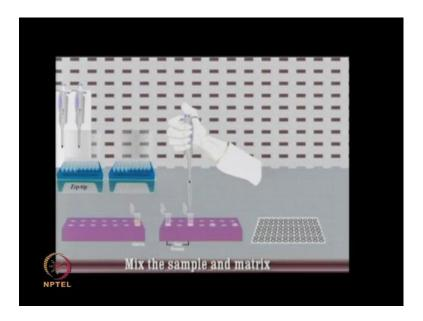
MALDI's perform in two steps. In first step the compound for the analysis should be dissolved in solvent containing small organic molecules known as matrix. This mixture is dried
