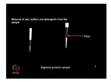
Once the protein sample has been digested all the salt buffer and any detergent must be removed from the sample. So, after doing in gel digestion and before proceeding further mass spectrum try analysis, in between an efficient step is to use some filters or zip tip which can eliminate some of these contaminants and salts. It offers several advantages such as quick verification sample embellishment and ensures that there is no contamination.
