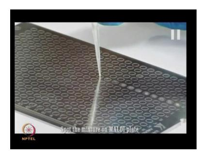
So, spot the mixture on the MALDI plate. How uniformly you can plate this mixtures on the MALDI plate ensure your good spectra and data quality later on.
