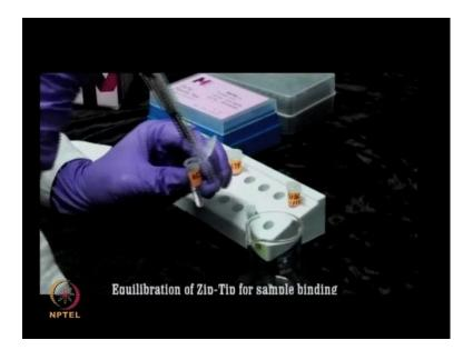
The in gel digested protein samples are further processed by using zip tip pipettes which contains c 18 or c 4 media for enrichment of peptides prior to m s analysis. Zip tip pipette tip within 10 microfiber pipette tip with a bed of chromatography media fixed at
