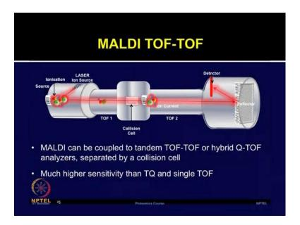
So, MALDI can be coupled to the tandem time of light in combination with another time of light. So, TOF-TOF or with hybrid quadruple time of light analyzers which are separated by the collision cells. Now for proteomic application it is recommended to use the TOF-TOF or q TOF the peptide ions are accelerated through the first time of light
