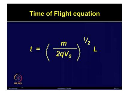
The time of flight of a charged ion can be calculated by using the equation shown in the slide. The flight time is directly proportional to the square root of mass of the ion. Now in this equation t represents time of flight, m is mass of the ion, q charge on ion, V 0 is accelerating potential and L is the length of flight tube.
