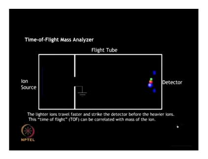
Fundamentals of MALDI-TOF ms. The time of flight analyser resolves ions, produced by the ionization source, on the basis of their mass to charge ratio.
