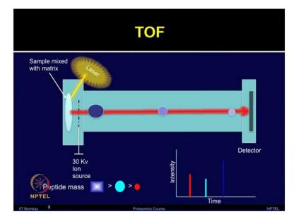
In time of flight tube the ions are accelerated to high kinetic energy, and due to the different velocities they are separated in a flight tube. As I mentioned earlier by adding the reflection on a reflector, the ions can turn around in the reflector that can compensate for minor
