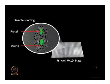
The components are mixed thoroughly and then the solution containing the organic matrix with embedded analyse of interest can be spotted onto a metallic MALDI sample plate. MALDI gives you an opportunity to analyse large number of samples in high throughput fashion.
