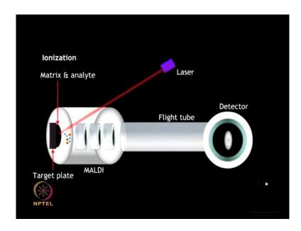
The target plate containing the spotted matrix and analyse can be further placed in a vacuum chamber, with high voltage and short laser pulse are applied. The laser energy gets absorbed by the matrix and is transferred to the analyse molecules which undergo rapid sublimation resulting in gas phase ions.
