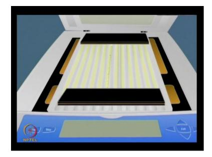
And then, move forward for the isoelectric focusing. So place the width at the either end of the IPG strip followed by an electrode at each end; fill all the adjacent wells with the mineral oil to ensure the uniform current flow. You can input the desired protocol on the instrument software along with the details of strip length, pH range, number of strips etcetera and start the focusing process.
