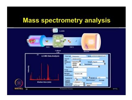
So, this slide gives you an overview of tandem mass spectrometry technique, and followed by how LC-MSdata can be analyzed by usingMascot search engine. So, different type of mass spectrometry techniques are available including Maldi-Tof and LC-MS based approaches and we will talk about these techniques in much more detail in the next module; we may talk about mass spectrometry.
