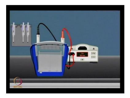
So prepare the gel casting solution consisting of acrylamide, bisacrylamide, tris chloride, SDS, APS and timid. Once the gel is polymerized then, you can add the IPG strip and now, ensure that assembly is properly sealed and buffers are properly placed so that proteins can be separated based on their molecular weight. Depending on the gel length, you can perform the second dimensional separation for few hour.
