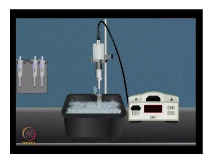
So presence of such high abundance proteins can interfere with the experiment. Therefore, we remove to we need to remove this high abundant protein. So, this experiment we tried both sonication and depletion of the high abundant proteins. After sonication is done then, we can add this serum sample on the columns usually these commercial available which can deplete various high abundant proteins.
