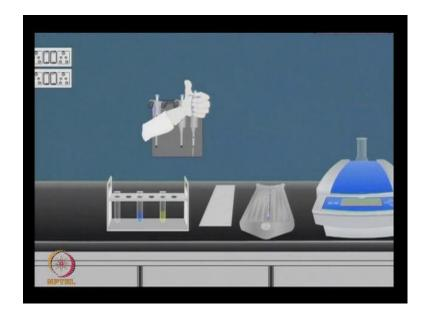
Now proceeds for the rehydration of immobilized pH gradient strips and focusing of these rehydrated strips. So remove the IPG strip form the cover, place it in the rehydration tray at the reconsidered protein sample on the strip, pour mineral oil to prevent it from the dry.
