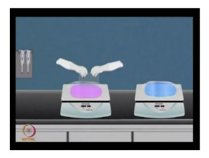
So this process involves removal of the gel from the electrophoretic assembly followed by treatment with a fixing solution, staining solution and finallythe distaining solution. You need to ensure that proper shaking conditions are maintained, and you need to allow 10 to 14 hours usually overnight strep for the staining as well as, distaining steps.
