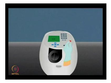
Once the color reaction has occurred then, perform the absorbance measurement at 595 nanometer. Once you have obtained good amount of proteins which was determined by the protein quantification.
