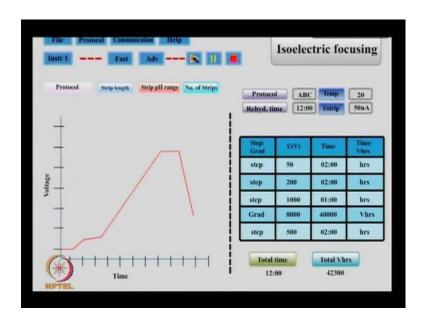
You can monitor the focusing progress on the software, and you need to ensure that focusing is proper. During the i e f proteins will migrate along its strip and come to rest at a point when there net charge becomes zero which is known as their iso electric point. After the i e f is done then, we need to separate the proteins in the second dimension on SDS page.
