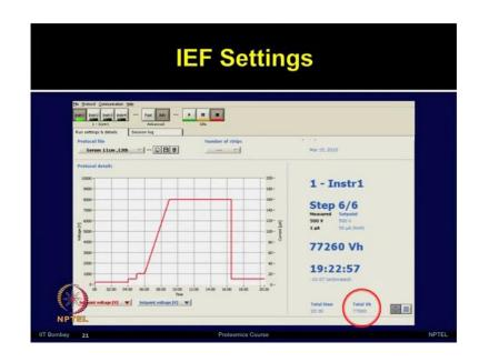
Now, when you are doing this serum protein separation the IEF becomes very critical because, you have lot of salt component in it, and if your salt removal is not effective, your isoelectric focusing run may not be very smooth. Sofor the software's you can monitor, how smoothly your isoelectric focusing is progressing.
