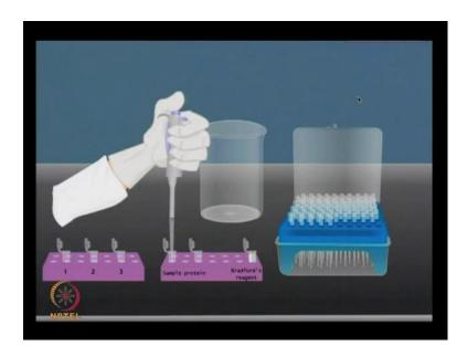
So, prepare the brat for dye region and label the tubes suitably for the standard and test samples; at these standard and sample solutions to their respective tubes. Now add the Bradford color reagent to the tubes and mix them thoroughly.
