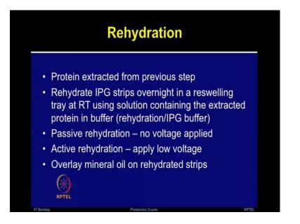
So, the rehydration is one of the important step before applying the electric field in the IEF process as you have seen in the previous animation, that to rehydrate the IPG strip you can apply the protein solution on the IPG strips. And different methods can be used for this whether passive rehydration, where no voltage is applied or active rehydration where you apply the protein sample and a very low voltage is applied to resolve the proteins.
