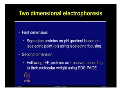
So, in the two dimensional electrophoresis the first separation occurs based on the isoelectric point of the proteins and the second dimension occurs based on the molecular weight. In the first dimension separation, you can separate the proteins in the isoelectric focusing unit, in the second dimension separation you can separate the proteins in SDS PAGE.
