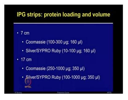
These are some recommendations for how much protein one should load on the IPG strips for example, if you have small strip like 7 centimeter length, you can apply between 100 to 300 micro gram of protein and maximum volume could be 150 to 160 microliters. Usually Coomassie stain is a good choice and if you have Coomassie stain
