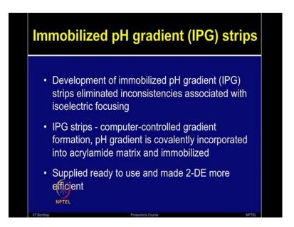
So, let us talk about immobilized pH gradients strip or the IPG strip, which was one of the major milestone developments in the 2-DE. So, the development of IPG strip as compare to the tube gel removed lot of inconsistency, which were involved earlier this is the process of isoelectric focusing.
