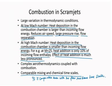
So, a such combustion in scramjets this is challenging because of the large variation in thermodynamic conditions you know. As I said before that you know gas turbine combustor it is as the flow is essentially conditioned by several things that is passes to a series of compressor blades rotor stator rotor starter plates and then it comes to the through the diffuser and they before then it goes into the to the combustor.
