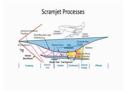
So, once again this to remind you these are the scramjet processes that which are of interest to us that if we are looking into the isolator and the combustor part that of course, we have a shock train and downstream of the shock train we inject the fuel. And the fuel must mix before it can burn and before it can burn there the fuel must ignite. So, mixing ignition burning these are the most important processes inside a scramjet combustor ok.
