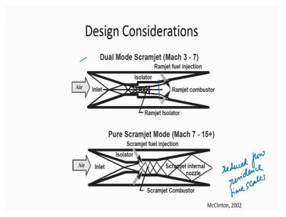
Then you have to have a range where it operates basically you can operate in a ramjet scramjet mode which is called the like dual mode scramjet. And then you can operate it in a pure scramjet mode when the mach number is greater than 7 ok.
