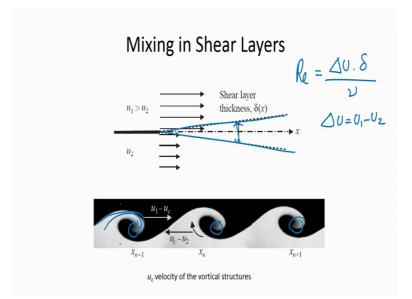
So, if we consider the mixing in shear layers. So, what is the shear layers shear layers is essentially that region in the flow which is characterized by strong velocity gradients and essentially which results in strong shear forces. And that is caused by when that is that happens when you have 2 parallel layers which are moving at different velocities as in this case.
