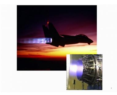
So, then we go onto this thing. So, this is how our flame in an afterburner look like. So, of course the aircraft is moving in this direction and the flame as you see goes out here and this is from a cavity engine afterburner that you see here. So, exact nature of the flame depends on the state of mixing, but here you see a blue flame. So, often the flame
