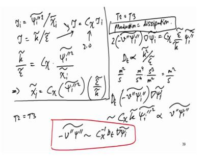
just like if you remember the integral time scale can be define like this. Favre average turbulent kinetic energy divided by the Favre averaged dissipation rate. And then this can be related by tau is equal to c psi by tau i whereas, c chi is typically taken to be 2.0 in commercial softwares and using this we can essentially model.
