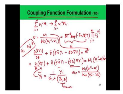
Now, coupling function formulation is the topic, and now we will consider a general reaction and general reaction, but a 1 step reaction because it is though it can be applied to multistep reaction it is easy to understand in terms of a overall 1 step reaction.
