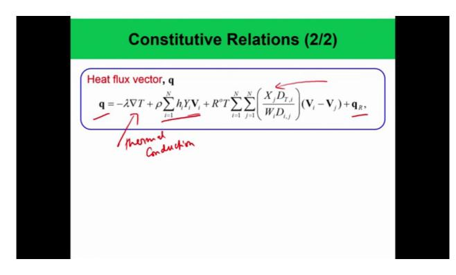
So, this will essentially we say that it can be able to neglect this part, and heat flux vector as we will see that this heat flux vector is given by this is the thermal conduction terms this is the thermal conductivity, and this is essentially the enthalpy transport this is the heat flux that is arising due to different heat contents and the diffusion velocity.
