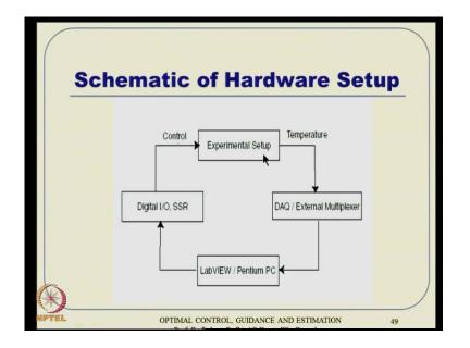
There are some hardware settings and this conceptually is like this. You have kind of experimental setup where you have to measure the temperature and there has to be some sort of I mean external multiplex sort of thing. Then you are pass it through this
