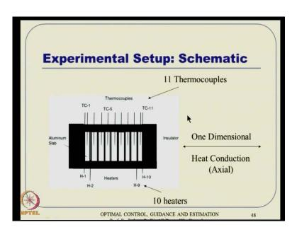
This is schematic of this. You have this eleven thermocouples, you have the aluminum slab; you have taken one dimensional heat conduction modeling sort of thing and they were ten heaters like that.
