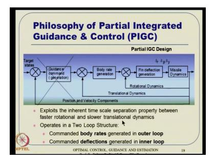
So, the idea is like this, we have this guidance but, you body rate spin deflection and all. What you are telling here is like come out of the typical guidance loop and whatever is left out is what your calling as partial IGC design actually. So, it exploits the inherent times scale separation property and then it operates essentially into loop not in really one loop but, we want to operate in two loops actually. And so, the commanded body rates
