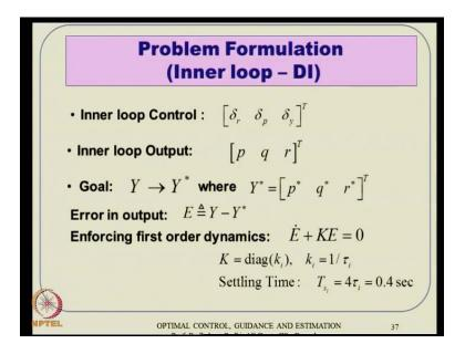
Then coming to inner loop control, we have this fin deflection and inner loop output something like this and the formulation y should goes to y star in the dynamic inversion sense. We define this error and enforces aero dynamic, K is diagonal matrix with diagonal entries been this one of the tau sort of thing actually. And settling time, how small we have assumed setting time have assumes as 0.4 seconds.
