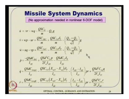
The equation of motion are given like that in involve in that it is complete full 6-DOF model. So, here is n dot, w dot, v dot, p dot, q dot, r dot equations, so this are quarter line components, there are gravity terms of this zee term are seen here. This are disturbance terms, which a difficulty to sum extent it is here known, something your known qualification known for that an then if we go back to dynamic learning (()) component and this quadrennial component.
