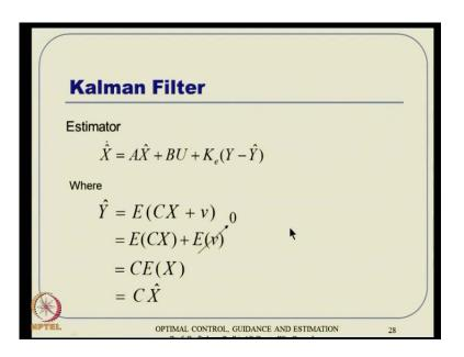
So, this is 0 and C is again expected value, the linear operator. So, C can come out and this turns out to be CX hat. So, Y hat is nothing, but CX hat. Even though definition tells that is expected value of CX plus V. So, you substituted back and present for that basically. That is what the message is here, ok. Now, what happens is this error co-variance matrix P of P is expected value of X tilde times X transpose there is like that one at before that.
