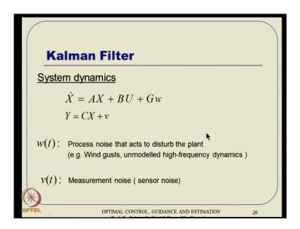
So, the system dynamics here we are talking about AX dot is AX plus BU plus G times w. That means, this is like a noise influence matrix sort of thing. This is control influence matrix B, but this is noise influence matrix. Remember process noise is a physical noise which is coming and acting on the system dynamics. So, that is the w of t which is process noise that acts on the system to disturb the plant actually, ok.
