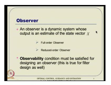
So, an observer is a dynamic system whose output is an estimate of the system vector x. That is the definition actually. So, essentially when we talk about why we got an observer, that what we are telling is we also got some sort of artificial system dynamics and that system dynamic output is nothing, but the state vector x actually, ok. Then, there ideas are full-order observer and reduced-order observer.
