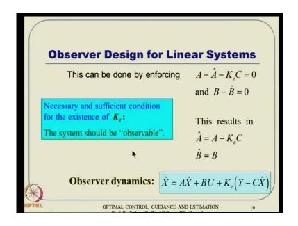
So, for that reason, we want to make the coefficients to be 0. That means, we got an expression for B hat and A hat from here. So, B equal to B hat and A equal to A hat plus K e C basically, sorry A hat equal to A minus K e C actually, ok. So, B equal to B hat and A hat equal to A minus K e C. Now, you substitute that till that K, this is my X hat dot. That is why started with only A hat and B hat was not known. So, now, B hat is B and A hat is A minus K e C actually, ok.
