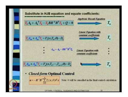
So, you do that and then you collect various coefficients, and coefficients of various powers of theta, and then... So, it happens that, ultimately it will resulting some times of Riccati equation, and this form and it will result in bunch of (()) equation rather, instead of Riccati equations, in terms of this series response actually.
