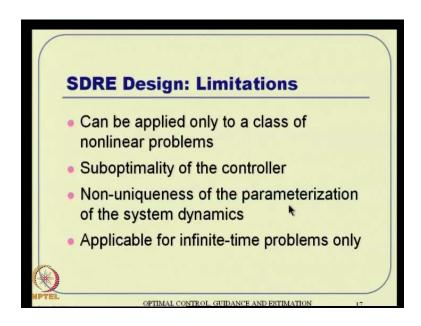
What are the limitations? The very first limitation is that it can be applied only to this class of non-linear problem that we are talking about, which is in general, true. Still, you should remember that, it is not a very universal non-linear control design that we can widely take and apply to any any non-linear problems actually.
