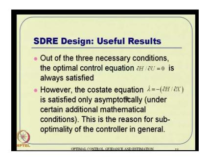
However, what happens to the vector problem. Now, the condition tells us that in in general in general, the vector for the vector problems, out of the three necessary conditions, the optimal control equation; that means, del H by del U is always satisfied, numeral 3 equations satisfied, state to state costate and optimal control equations.
