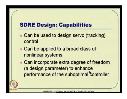
So, it can also be used for tracking control applications, thus that you can see that in a couple of slides later. It can be applied to a broad class of non-linear system that is, what we are talking is, this control fn system and stc parameterization, where a of x has certain certain nice properties that is not a very restrictive class of non-linear system, and many problems including aero space problems, as well as a robotic something like that, it can be actually model it that way.
