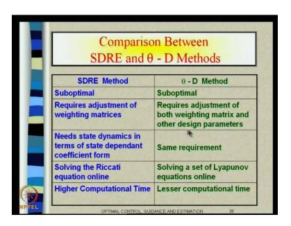
So, in summary there is a small comparison thing that you can think about. On one hand, we have A SDRE method and on the other hand, we have theta D method. Both are applicable for control affine systems only and do not forgot actually, and both lead to sub optimal solution. This require adjustment of weighting matrix and Q of x r of x actually,
