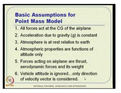
So, basic assumptions for point mass model. First of all, we are all kind of collapse in the entire vehicle at the CG of the airplane; that means, all forces act on the CG of the airplane, then the entire vehicle is just a point; and acceleration due to gravity is constant. We are not bothered about variation of g, unless you talk about very long very kind of inter-planetries missions something like that, when you really go far away from earth actually.
