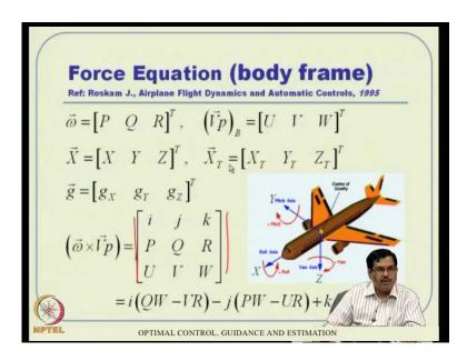
So, before you, I mean before we move along, we will decompose this. Now, we will decompose this vectors notation into components now. So, this entire rotational rate consists of P, Q, R; P is about X axis, Q is about Y axis, R is about Z axis like that in the body frame. Similarly, V P the total velocity vector will have U, V, W component; the
