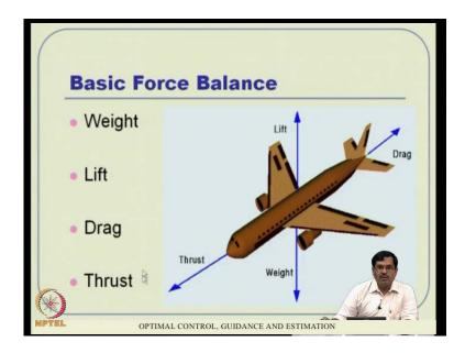
So, any flying object in a straightened level flight, let us say, tries to contract to this forces gets generated and balance each other actually. First thing is, there is a weight component, which is vertical. So, there must be a force, which is upward, which should contract that actually.
