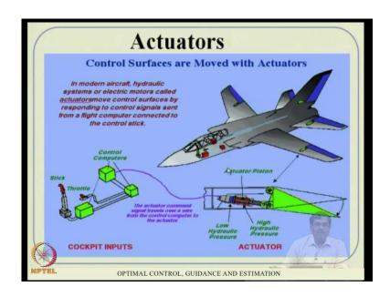
So, that is ultimately executed through actuators, actuators will be situated, now modern day aircraft actuators are situated right there, where you really need that and the command, as everything goes through all sort of computation through, through a flight computer and essentially, the signal is transmitted through a wire to this, this actuator system actually actuates the system, it deflects that, that aileron, for example.
