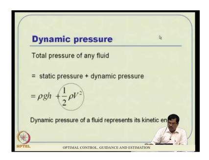
Now, coming to the dynamic pressure part of it and what we saw here is half of this dynamic pressure and this dynamic pressure is actually, you can visualize, the total pressure of the any fluid is partly from static pressure and partly from dynamic pressure, and the static pressure is rho g h (()) potential energy sort of thing. And then, there is a dynamic pressure, which is essentially kinetic energy content actually. So, this is what plays a role in generating lift and drag essentially.
