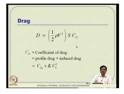
Now, coming to the drag part of it, the drag is also given by very close formula. Instead of C L, what you replace is C D, but also remember, that C D is roughly a function of like this, a function of CL in a, in a quadratic way. So, C D is, essentially, C D0 plus KCL square; that means, it actually varies in a quadratic manner always.
