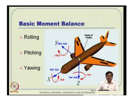
So, the basic the moment balance is, essentially 3 moments are there, one is rolling moment, another is pitching and another is yawing essentially. This, this is something called body axis actually, you can visualize an axis frame setting on the central gravity of the vehicle, where x axis is pointing to the nose, y axis is to the, what is called as, star board, right side of the, thing, wing and then, there is like, the vertically down is something called z axis actually.
