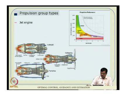
So, jet engines can be classified into like turbo jet, turbo flow, turbo fans, and things like that and this is roughly the behavior what we expect actually, I do not, whether this, this slide is not very clear. So, what is plotted out here is Mach number versus specific impulse ISP and this ISP, this is, by definition something like thrust by mass flow rate actually.
