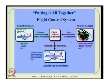
So, in a nutshell putting it altogether, there is a flight aircraft sensors, which will sense the measurements and then pilot command also pilot will see outside and all that, that also you can, that a huge amount of sensor, that goes through pilot organs basically, like I, sort of things then, he gives a command essentially, that, that also counts to the control computer. It goes through a variety of computation, then it gives a control command, which is essentially executed there.
