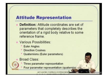
So, let us see that, so Attitude Representation by definition is essentially the attitude coordinates are set of parameters that completely describe the orientation of a rigid body
