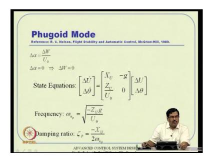
So, under these assumptions delta alpha become 0 with alpha remains constant and with delta alpha delta alpha is defined that way. So, delta W also becomes 0, so you are left out with this nice small matrix and I mean homogeneous linear system which you can analyze it very clearly, this is a second order system in a way delta U and delta theta you have to analyze together basically.
