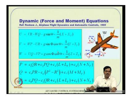
And then we went out and derived this set of equations, which essentially consists of a translational oscillations and rotational oscillations terms actually, and this consist of partly this carioles component and partly from gravity and partly due to external forces and similarly, you have this equations of for rotational rates and all that actually. So, we have done that in detail in previous class.
