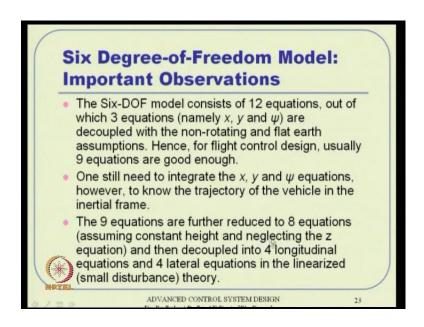
Now before you go ahead there are further comments. First thing is six of models consists of 12 equations out of which 3 equations are decoupled with the assumption that the earth is non rotating and flat like thing, like what I told also last class if you see all those equations essentially the psi actually, and then X Y do not come in any of the rest of the equations actually.
