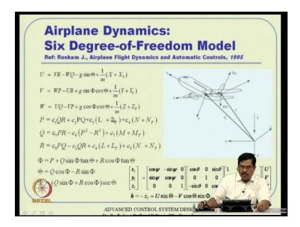
So, which is here, so you see this consist of U dot V dot W dot P dot Q dot R dot then finite theta dot psi dot and then X I dot Y I dot Z I dot. So, this 12 equations we will derive that and normally this height dot this s dot is actually negative of Z I dot that is, if you simply take out the last row and make a negative sign, then it will provide a and nothing but X axis.
