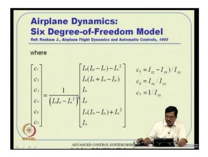
And then I mean if you go and see that this c 1 and c 2 all these things we saw that last class also, whatever c 1 c 2 c 3 I mean all this c with a suffix what you see here in P dot Q dot R equations are essentially functions of moment of inertia which is which is given like that actually.
