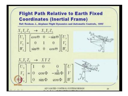
Then we have this next transformation by angle theta. So, this angle theta is with respect to U 3 and W 3 remember that, because Y axis remains fixed here, so V 2 is equal to V 3 but the other variables U 2 V 2 W 2 is related to U 3 V 3 W 3, because of that actually because of angle this rotation angle theta and similarly, this X 3 Y 3 Z 3 goes to X Y Z by angle phi ultimately. Now this is a rotation about X axis actually the transform X axis.
