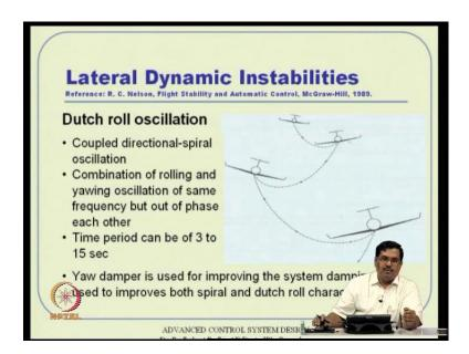
And then there is a nice coupling with the 2, this what is called a Dutch roll oscillation. So, here it is it will the directional spiral oscillation should be coupled together actually. It will roll and hence it will beta will be low it will go somewhere then it will stabilize.
