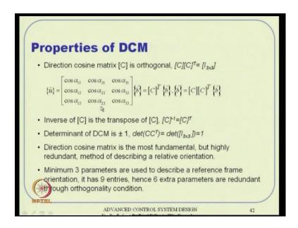
Now before do that before even talk about that, let us say observe some nice property, that C is essentially an orthogonal matrix and orthogonal matrix is a nice property the C time C transpose is actually identity, that means inverse of this matrix is transpose and inverse is all
