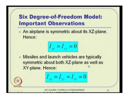
Then also remember, that airplane is symmetric its one of the assumptions. So, that is why this cross moment are 0 and missiles and launch vehicles are typical symmetric about both the both X Z plane and X Y plane and hence all the three cross moment of inertias are here.
