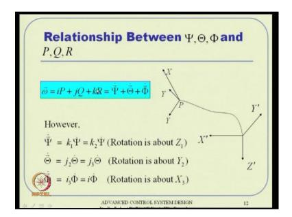
So, how do they vary actually? Now obviously they are related to in this body related rotations P Q R. So, if phi theta psi is what this inertial coordinate frame rotation in a sequential way.
