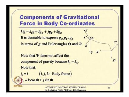
So, if you let us try to quickly do that and this essentially, the same way remember gravity is perpendicular to the I mean parallel to the initial Z axis all the time, no matter whatever is the vehicle attitude gravity is always vertical with respect to surface of attitude only. So that means it is always parallel to the Z axis it is always pointed to the center actually earth center.
