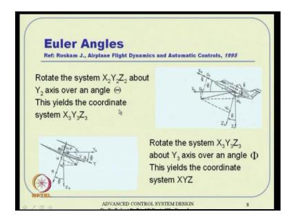
And the next what you will do is this rotated frame whatever is this you rotate it by angle theta about the Y axis. So, first with respect with Z axis then with respect to Y axis and ultimately with respect to X axis phi that is what you will do here.
