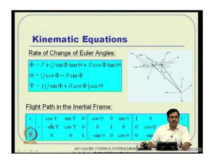
So, this is how the entire six of equation is made up, but before going there, so last previous lecture, we have seen the dynamic level equations, here we see that kinematic level equation. That means velocity level equations, these are angular velocity term and these are the translational velocity terms. So, this 6 equations couple with the previous 6 equation what we say that last class derived the complete set of 6 equations.
