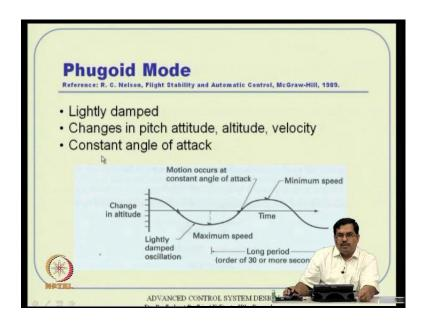
So, one thing is which is which is called as Phugoid Mode, sincerely the aircraft drops its height to a significant thing and then goes up actually the vehicle attitude does not change the attitude remains same the entire vehicle will keep on going and then coming down an then rise like a roller coaster ride actually. So, this happens with something like constant angle of attack actually.
