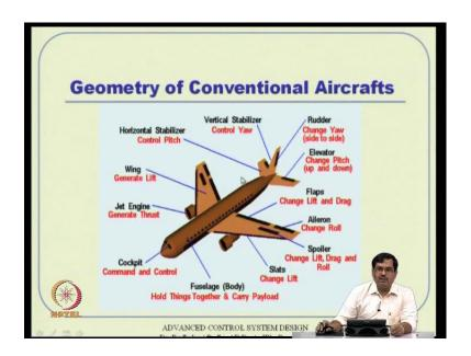
Now coming to the conventional aircraft geometry, if you see the aircraft geometry there are various parts of the aircraft that is specific requirements. It is a complex system of course. It is first of all engines which is required for propulsion, it has a huge fuse law sort of thing where people can sit, move around and things like that. That is where people sit two wings here which largely are responsible for this generating lift.
