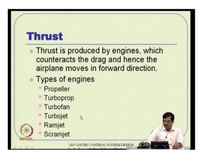
Now coming to the thrust force, so you remember there are we talked about weight lift, weight versus lift and drag versus thrust. So, this thrust generation happens through variety of through variety of ways and you have to essentially use an engine to do that. And it can happen through a propeller through a turboprop, turbofan, turbojet, ramjet, scramjet in a variety of things which are field by itself.
