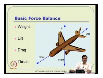
So, any flying object in a straightened level flight, let say has to counter act I mean this four forces get generated and they balance each other. First thing is there is a weight component which is vertical. So, there must be a force which is upward which should counteract that. So, there is a weight which is balanced by lift, but this lift generation mechanism also
