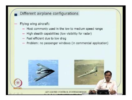
Then, there are various other designs. This is something called flying wing aircraft. That means, you can visualize the entire thing as a single wing and these are all requirements from stealthy considerations. It is a high stealth capability that is low visibility to radar. Fuel efficient, it is also fuel efficient due to low drag. Typically it flies at very high altitude. So, the air density is very low, dynamic pressure is low, drag is low. We will see that just little couple of slides later.
