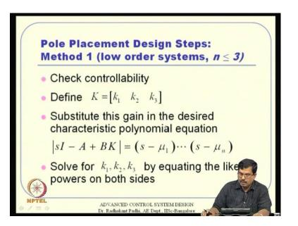
And, this turns out to be like not a very convenient method, but if n turns out to be less than equal to 3 sort of thing, may be to 4 maximum. Then, we can certainly go ahead and equate these polynomials... And then you can, we should be able to solve this k 1, k 2, k 3 directly, basically.
