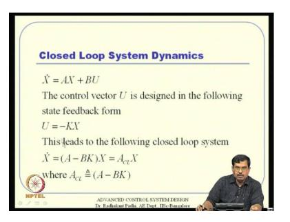
Then, there is an idea of closed loop system dynamics. So, these are all, when something is given like this, it is open loop system for say. And then, if you come up with a control design U in the form of state feedback, in other words U is equal to minus K X.
