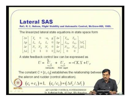
So, what is about lateral stability augmentation system? It is something like this. Very similar, very parallel, actually. So, this is v, p, r and phi. If we put them together, but the problem here is this is like both of the control that is... are equally effective; that means they are equally fast actually. So, I cannot neglect the one over the other for sake.
