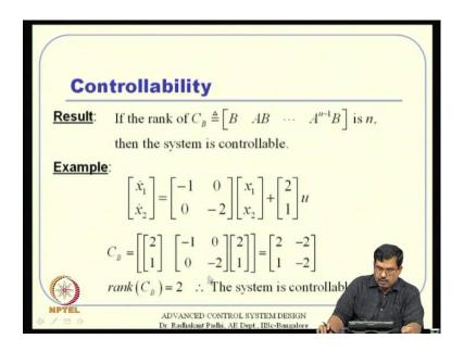
So, then coming to controllability; before we design any control system, we need to check controllability. And, for linear time invariant systems, the test is very straight forward. So, we just formulate this controllability matrix. And, if the rank of this matrix is n, then the system turns out to be controllable.
