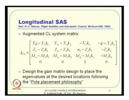
So, when you do this A minus B K, then A minus B K turns out to be like this. So, you have this B times K; B is here, B times K is a matrix say 4 by 1, this is one by four. So, it will turn out to be four by four.
