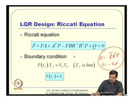
So, this Riccati equation if it is solved, then it is and we will be able to get that t. That t will be used for lambda. And once, you get for lambda and then we got this minus R inverse B transpose B times X. and hence, R inverse B transpose P will turn out to be the real matrix actually. So, but for solving lambda, I mean solving for P we also see the boundary condition. And, this boundary condition what you see here, if you utilize that you will get this kind of boundary condition.
