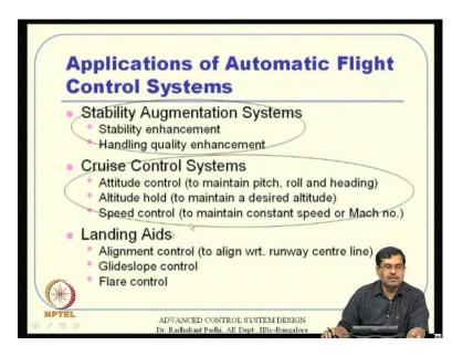
So, last class we also saw that application of automatic flight control systems can be many. I mean applications of control theory for automatic flight control system; that is what we are talking here. And then, largely you can categorize them as three to four categories.
