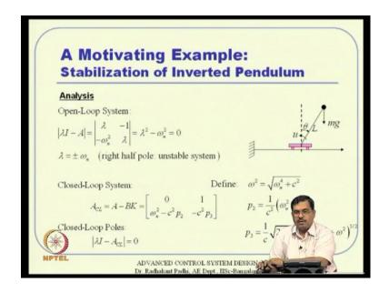
So, now the question is we got the solution is there any guarantee that. So, I mean this particular controller needs to be stabilizing controller let us examine that question. So, first we analyse the open loop solution open loop solution remember considers-considers only this a matrix whatever a matrix is there here without any control term control is zero.
