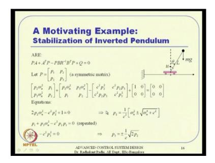
Now, let us go to the r e algebraic Riccati equation solution. So, this is our equation P A plus a transpose p minus B P R inverse b transposes p plus q equal to zero. So, we have all the matrix elements ready now a b q r all that put it back and also remember we want a symmetric positive definite solution for P ultimately.
