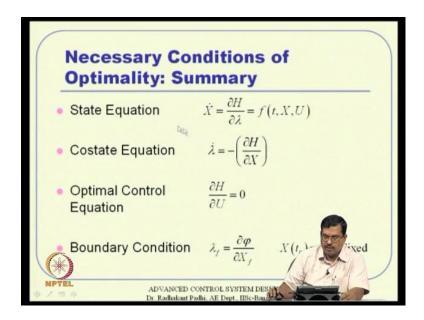
And associated with these four problems, we also went ahead and derived these necessary conditions. So, essentially it talks about three path conditions and one set of boundary conditions actually. So, path constraints one is I mean two of them are dynamic equations one is state equation, and there is cost ate equation and associated with that there is optimal control equation which needs to be satisfied at all point of time. So, that is del H by del U equal to 0.
