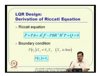
So, that is how we we tell that this coefficient matrix has to satisfy this constraint that is this P dot plus P A plus a transpose P minus PBR inverse B transpose P plus Q equal to 0 which is commonly called known as Riccati equation all the this differential term here P dot. So, it is also called differential Riccati equation actually.
