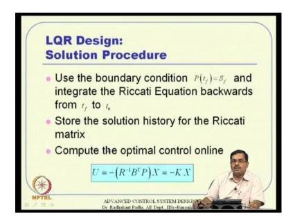
So, starting from t f we can make use of this equation and then integrate this equation back work. So, that we can get a solution of P of T at every point of time and we can store that P of T we can store the solution history for the Riccati matrix and then we can compute the optimal control online by using this relationship ultimately.
