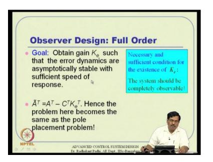
And as I told, the goal here is to design K e such that the error dynamics are asymptotically stable. And also remember that we have to have sufficient speed of response, because there is the whole idea is to decay this the error very fast; and and then you can do that, because we are not talking about a controller design, the control effort is a physical effort, here is all numerical actually.
