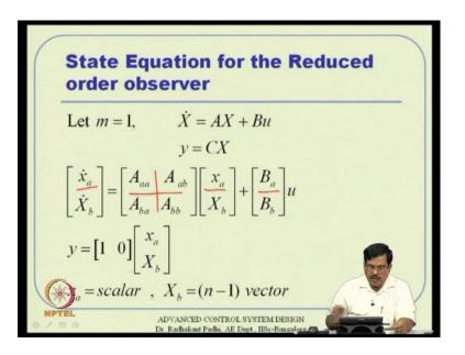
So, let us study this in slightly detail. So, what we what we are asking here is, we confine ourselves to m equal to 1 that means we have a like single output getting measured actually. So, that is what we want. And then without loss of generality we want to put that it is the first state in the state order, we just tell the we just we are claiming that, the state vector X is partition into this small x a, which is a scalar and the big X b, which is a vector.
