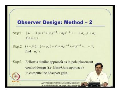
So, obviously we do have a better technique that is the method 2. That is what we talked last, that is a Bass-Gura approach of control design as in a pole placement control design. So, we will take the advantage of that approach. And then, first design K e transpose and then take transpose of that to get K e. So, the let us talk about that.
