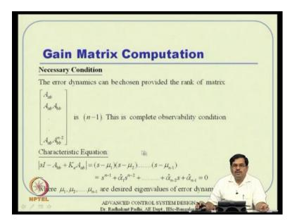
So, again the necessary condition is given in terms of observability matrix for the reduced order system in case. So, reduced order system observability matrix turns out to be like that; and this way rank has to be n minus 1, now because 1 is gone actually form there, (x, y) is not part of the output part of the state equation. So, what we need is, the rank of the matrix should be n minus 1 actually.
