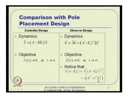
This is very similar to what we had it in controller design can see controller design what that the this was our dynamics, where U equal to minus K X, so A minus B K times X. And the objective was to drive X to 0. Here the dynamics is like that, that is what we got it actually, the dynamics is like that. And then, the objective is to go drive E to 0.
