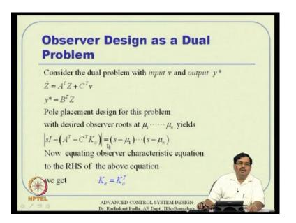
Now, as we discussed in the last class, there is a nice concept of duality we know that. So, if you consider this is a dual system of like this Z dot equal to A transpose Z plus C transpose v, where v is a virtual control input. And then y star is B transpose Z; then we know that, this the controllability of this turns out to be observability of the original matrix. And that is how it appears here also A transpose minus C transpose K e transpose actually here (Refer Slide Time: 15:53).
