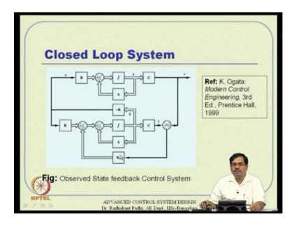
So, the closed loop system I mean block diagram sense it will operate that way. So, u will get computed from X tilde through minus K this is nothing but the control gain actually whatever gain you had. But this u will act both on the on the actual plant and it will also act on the observer plant actually. This this lower side of that is observer plant, the upper side is the control plant actually.
