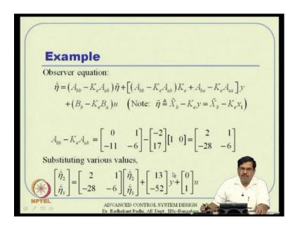
So, we have to find out an observer equation also and this is the formula again we substitute various values. And of ultimately we see that, this is my reduced order observer dynamics. So, I start with some guess value for eta 2 and eta 2 tilde, and eta eta 3 tilde; and I keep on propagating this equation along with some I mean some control which is like minus K times X basically.
