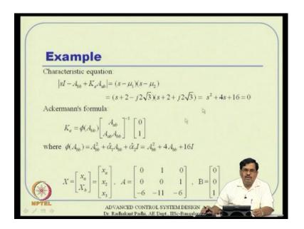
So, then you can go back and substitute your characteristic equation turns out to be like that, remember these are all partition matrix, small smaller dimensions than what you had originally. We put that in characteristic equation, then expand it and you will get s square plus 4 s plus 16 which is equal to 0. That means you you collect the the A 1, A 2 from there and then you have a Ackermann's formula you can directly use using this way.
