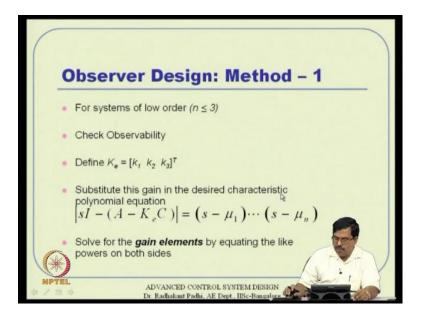
So, that is what a method 1 tells about. So, if it is n is less than equal to 3, then first thing you need to do is check observability. And if the observability condition is satisfied and let us assume n equal to 3 here, then define  $K \ 0$  K e is nothing about K 1, K 2, K 3. Remember the control gain, where control gain matrix was a kind of a row matrix I mean row vector. And observer thing, the gain is these kind of a column vector actually that will be (()) from equation itself actually.
