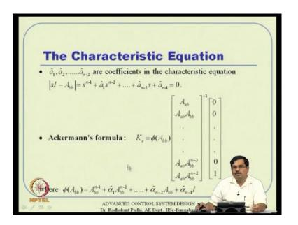
So, all these tools are available to us say already to us actually. Again the same separation principle holds good nicely (Refer Slide Time: 46:08), where you can show that the the poles of the overall system are nothing but about poles of the poles due to pole placement controller, and that is poles due to reduced order observer.
