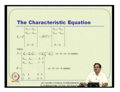
And you get this is method 1, you can directly equate to the characteristic polynomial. Method 2, you can equate through the Bass-Gura formula, where W is given like that and tilde is your reduced order observability matrix or you can have a Ackerman's formula also we can we can directly use it in the formula sense. (Refer Slide Time: 45:57)
