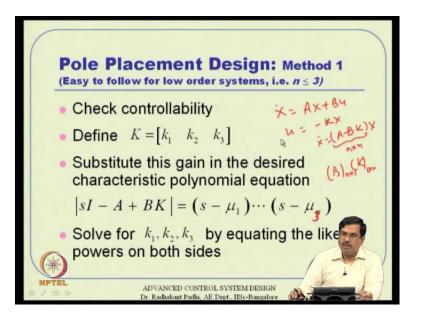
So method one: That is what we talk about so far. The very first step of any control design, not necessarily pole placement is check controllability. Once the controllability condition is satisfied, then there are further is hope that you can actually design a controller otherwise no.
