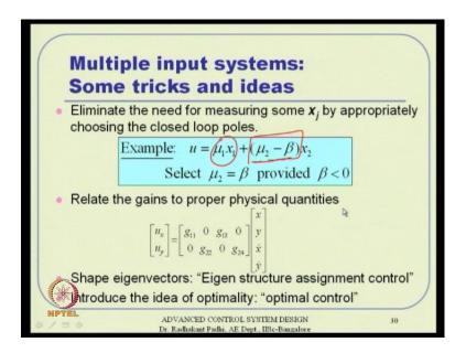
So one idea is you can eliminate the need of measuring certain x certain states by purposefully selecting some sort of a combination. Appropriately, choosing the closed loop poles. For example, if your control formula in a symbolic sense is like this where, mu 1 and mu 2 are pole locations. Then purposefully I will select 1 mu 2 equal to beta. So this term equals to 0 and hence I do not need to use x 2 I do not I can eliminate sensor.
