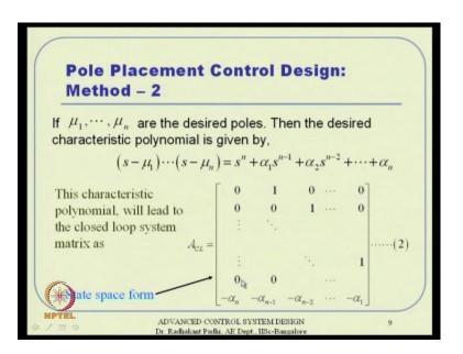
Now if we have the close loop pole locations known to us and that is s minus mu 1 multiply s by s minus mu 2 all that up to s minus mu n. Then, it will result in a characteristic polynomial and this characteristic polynomial will lead to a closed loop system matrix in this form.
