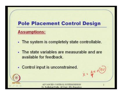
So, the assumptions behind this particular design, first thing is the system is completely state controllable. So, if it is not controllable obviously, you cannot do anything and hence we cannot do pole placement design either.
