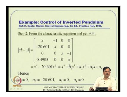
So next go to the step 2. This is what we are talking about, like a practical example of a using our theory what you know. So s I minus A is nothing but, the open loop characteristic polynomial A matrix is like that, A matrix is given like that. So s I minus A turns out to be like that. And s I minus A determinant turns out to be just these two terms s to the power fourth and s s square.
