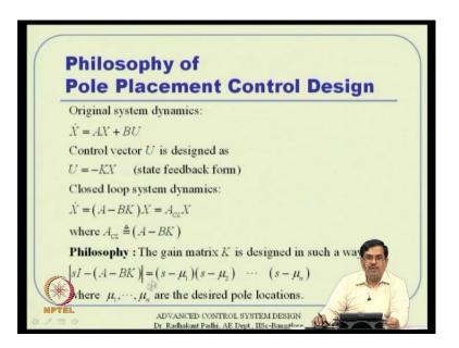
Now philosophy of loop what is the idea there? What is the philosophy of pole placement control design? We have this plant which is I mean X dot equal to A X plus B U linear system dynamics. And we want to design a control vector U, in the state feedback form. That means U equal to minus K X.
