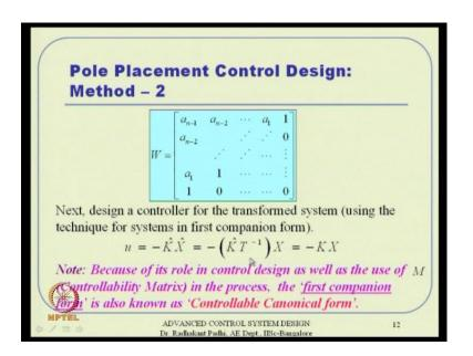
Initially you have a matrix I mean coefficients which are nothing but, coefficients of this characteristic polynomial if it is in the kind of first companion form, or the in general otherwise it will have this a 1 a 2 all this a n will come from the open loop a matrix actually. We will see an example to see, how do we select this and all that actually.
