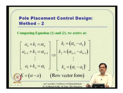
So then you result this set of equations will pop up and from which we will be able to compute k 1 to k n very easily rather. So in a vectorial notation K is nothing but alpha minus a where, alpha is a row vector containing alpha 1 to alpha n and then a is a row vector containing a 1 to a n actually.
