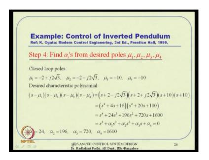
We have to find this; we have to also cater for this desired close loop like a poles and all. And desired close loop poles are given like that. Also remember for real characteristic equations are typically real polynomials. So the closed loop pole locations, the only restriction that to select is they have to be complex conjugate. If they are complex number they have to the conjugate pair it should exist actually.
