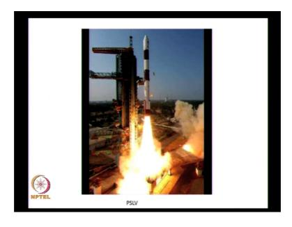
This is our PSLV; Polar Satellite Launch Vehicle of India again. And here, again you find straps around the first stage - you have straps. Six straps or four straps could be put. Then, you have the second stage, third stage.
