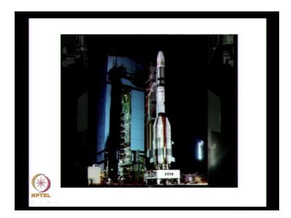
And, this is the GSLV. As we just now saw, these were the four straps. This is the first stage, second stage and the third stage. First, these four stages are ignited. Four straps are ignited, gives you the thrust to take off. Immediately after takeoff, the core is also burning. Therefore, you have the huge thrust which pushes it. Then the second stage fires, then the third stage fires. And, this is how a rocket functions.
