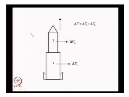
We go through a few slides. You know, here we see a two stage rocket. May be the first stage gives you a velocity  $\Delta V_1$ , the second stage gives you a velocity  $\Delta V_2$ . The total velocity of this combination of the first and second stage is  $\Delta V = \Delta V_1 + \Delta V_2$ . This is a two stage rocket.
