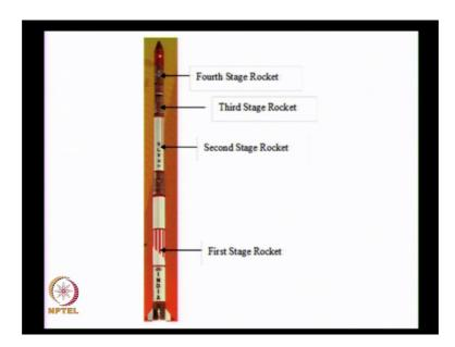
Let us go to the next one. This is the first rocket which was designed in ISRO at Trivandrum. This was in the period, may be nineteen seventy to seventy eight. And, the first successful launch was in 1980. It was a simple rocket, you know. It consists of four
