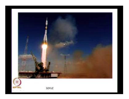
This slide shows "SOYUZ", a Russian rocket. Here you have straps here or a cluster of engines here and the main engine is firing. The exhaust from the several rockets is interacting to give the shape of something like a ball. And, "SOYUZ" was used for launching our first experimental satellite namely "Aryabhatta". This was in nineteen
