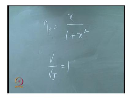
Now I want to ask you, when will the propulsive efficiency be a maximum. Just look at this expression. Just be unbiased and tell me whether I can identify a condition for the propulsive efficiency to be a maximum. We will anyway solve for the maximum. We will find out the maxima and get the condition. But, by looking at this expression can you tell me when should the efficiency become maxima?
