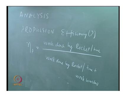
We would like to know what is the efficiency of a rocket. What do you understand by efficiency? We are looking at the rocket flying up; therefore I want to find out how
