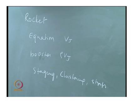
Well, I think by now we should be very clear about what is the principle of rocket, what is the rocket equation as it were, what will be the rocket equation modified for a booster, in which case rho  $V_J$  becomes more important than  $V_J$  itself. And then, we talked in terms of staging, clustering or and also straps.
