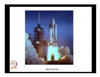
This shows the Space Shuttle taking off. These are the two boosters. Solid rocket straps as I said and you have three engines which generate the thrust.
