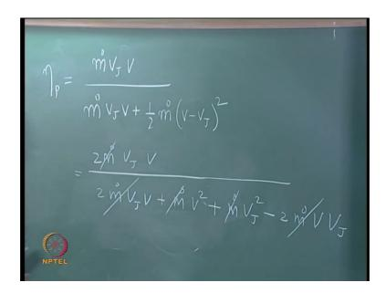
And therefore, how will I put the expression for propulsive efficiency together? I will now write the efficiency as  $\eta_p$  (propulsive efficiency) is equal to the useful work done equal to  $m^\circ \times V_J \times V$ . This is divided by useful work  $m^\circ \times V_J \times V$  + the kinetic energy per unit time viz.,  $\frac{1}{2}$   $m^\circ \times (V - V_J)^2$ .
