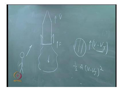
Let us try to sketch the factors involved. We have a rocket going up. It goes with the velocity V. It is pushed up by a force. Therefore, the useful work which is done by the rocket is the force into the velocity per unit time. In the process is anything getting wasted? What is the waste? How do we get the waste energy or work?
