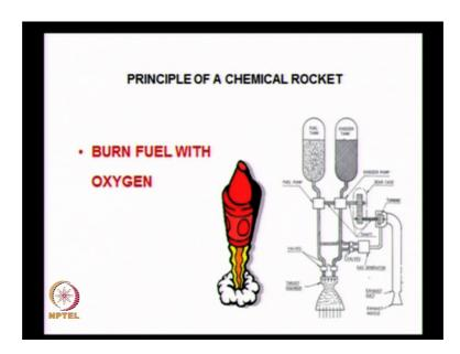
What does a liquid propellant rocket consist of? We are yet to study it. You have a fuel tank, you have an oxidizer tank, you pump the fuel and oxidizer into it, you ignite it and you push the gases out. So, this small insect which is available in nature works on the principle of a liquid propellant rocket or rather the rocket works on the principle of the bombardier beetle.
