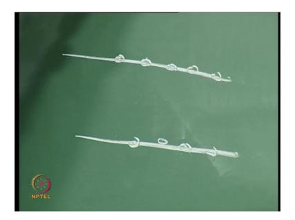
But shower head injector is something like a weak injector, because as you know the jets formed are all parallel. It takes some definite time for it to atomize and form droplets, but you want droplets as early as possible. Mixing of the fuel and oxidizer is also difficult.
